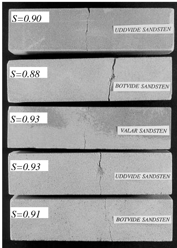
Figure 3.8.3. Damaged stone prisms ( 3 \times 3 \times 12 cm) after S_{crit} -test with high degrees of saturation according to the freeze-thaw cycle shown in Figure 3.8.2.
