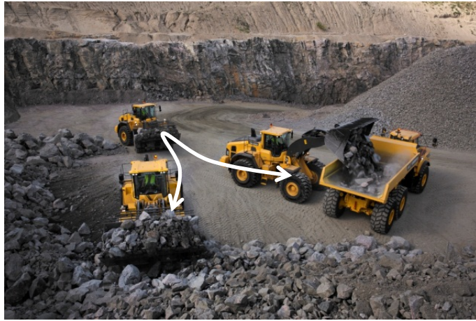
Fig. 1.1 A wheel loader performs a "short loading cycle" in blasted rock from face as a part of a production chain. Modified from [19].
