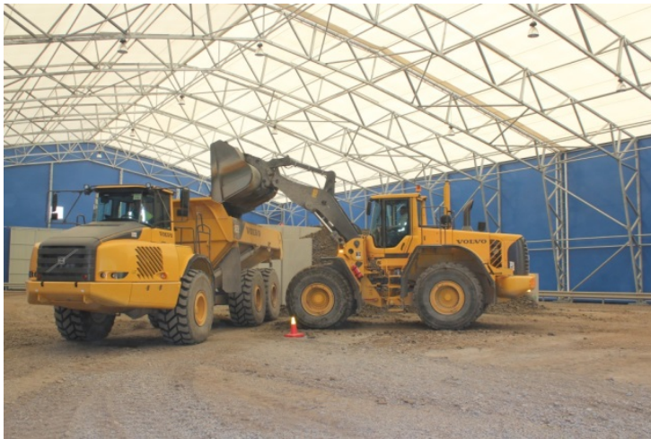
Fig. 4.3 Measurement setup; loading gravel onto a load receiver in a “short loading cycle”. From Fig. 2.1 in Chapter 2.
