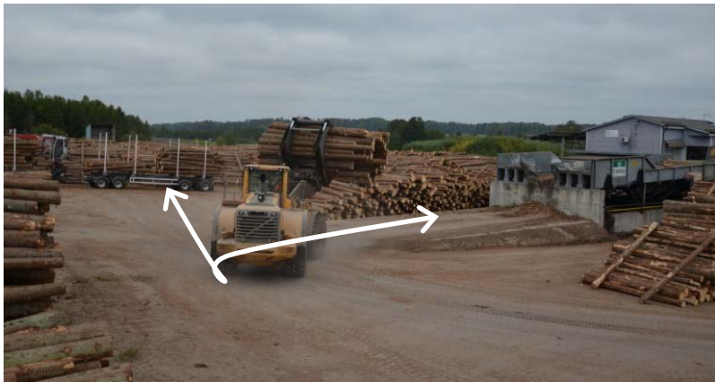
Fig. 4.5 A wheel loader with grapple, unloading timber from a truck to a sorting table.
