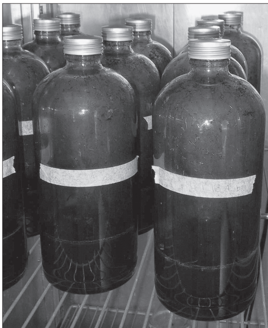
Figure 1. Reactors for determination of methane potential (2-litre glass bottles with septum corks).
