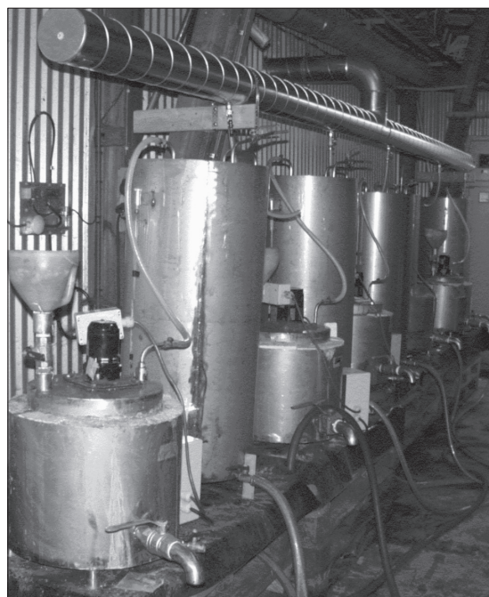
Figure 2. The systems for pilot-scale continuous anaerobic digestion.
