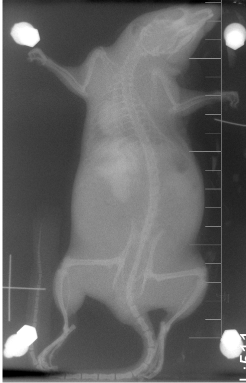
(a) A one-minute exposure of a sacrificed Wistar-Furth rat ( \sim 2 cm thick). The grey scale extends from 2 \mu\text{Gy} (white) to 13 \mu\text{Gy} (black). The image is 20 cm high.
