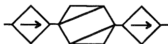
Figure 3.22 One flow structure describing the pump and valve. The pump and valve are modeled as separate transport functions. The balance must be present for syntactical reasons. In this model, the pump and valve may be conditioned by different subgoals.
