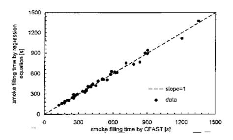
Figure D2. Result of regression analysis for non sprinklered fires
