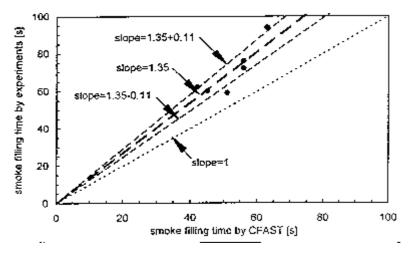
Figure D4. Comparison of smoke filling time calculated by CFAST with full scale fire experiments
