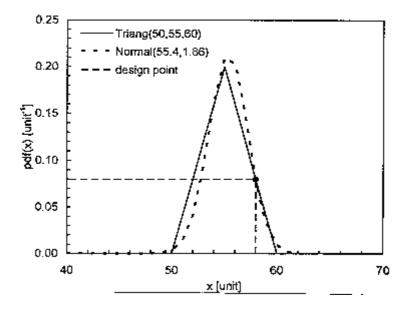
Figure C4 Triangular distribution and corresponding equivalent normal distribution
