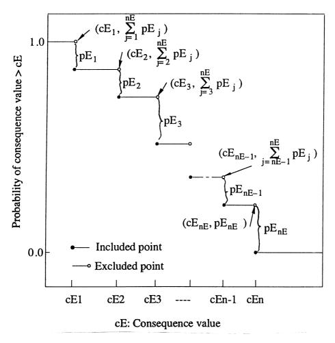
Figure 7. Construction of a CCDF [6]
