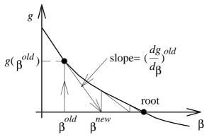
Figure C1 Newton's iterative method to solve  $g(\beta) = 0$ .
