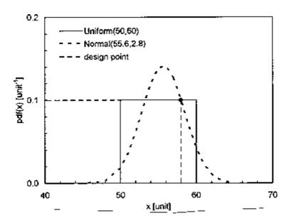
Figure C3 Uniform distribution and corresponding equivalent normal distribution
