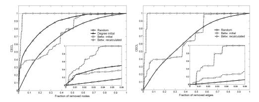
The node and edge-based removal strategies are very similar for both Systems A and B. This is due to the fact that the systems are mainly radially fed, *i.e.*, most nodes have a degree of two. In the remaining part of this paper, we focus on node-based removals, but much of the discussion is equally applicable for edge-based removals.
