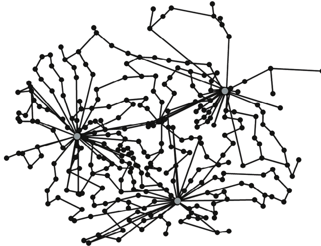
Figure 3. Overview of the electric distribution system. The larger circles indicate in-feed nodes and the smaller circles indicate load nodes and transfer nodes.
