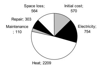
Figure 6.14. The different components of the LCC in SEK/m<sup>2</sup> excluding VAT for the example in Section 6.2. The area in the denominator is  $A_{BTA}$
