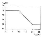
Fig. 5. The supply air temperature,  $t_{SA}$ , as a function of the outdoor temperature,  $t_{out}$ , with the control strategy called "decreasing" and the temperature coordinates (10, 18) and (20, 21).
