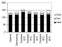
Figure 12. The calculated annual energy use for the simulated office zone in Kiruna, North Sweden, per floor area for different supply air temperature control strategies. "Cool" relates to  $P_{cm}$  "Fan"  $P_{fon}$  and "Heat"  $P_{rod} + P_{boil}$ .
