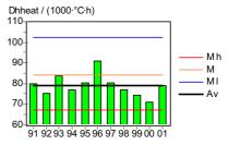
Figure 10. Annual degree hours for heating for the readings for each year respectively together with the average from the extreme and normal years of Meteonorm for Lund.
