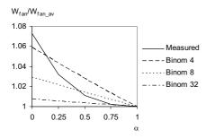
Figure 20. The ratio between the energy use for the measured or simulated case and the energy use if the average airflow rate were used for calculations. The simulated distribution was binomial with  $p_{pin}$  according to the average from the measurements but with a different number of rooms. Equation 17 defines  $\alpha$ . The data is for the municipality planning office and daytime.
