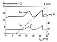
Fig. 10. Optimal supply air temperature  $(t_{SA})$  and supply air flow, q, at different outdoor temperatures  $(t_{out})$  and with a constant load,  $P_{load} = P_{internal} = 200 \text{ W}$  (U = 0) corresponding to 15 W/m² floor area.  $\eta_1 = 0.5$ ,  $q_{min} = 16 \text{ Us}$ . The dashed line is the saturation temperature  $(t_{sat})$ .
