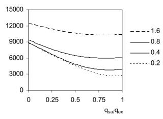
Figure 3.8. The annual energy use for heating all incoming air for a typical detached house located in Malmö depending on the ratio between supply airflow rate and exhaust airflow rate. The exhaust airflow rate,  $q_{ex}$ , is set to 70 l/s. The ratio between the supply and exhaust airflow rate is varied. The legend shows the specific leakage in l/(s·m²) at 50 Pa pressure difference. The Swedish building code (Boverket, 2002) sets the maximum limit to 0.8 l/s for dwellings.
