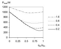
Figure 9. The total power for heating the air at default conditions. The legend gives  $I_f$  in  $1/(s \cdot m^2)$ .
