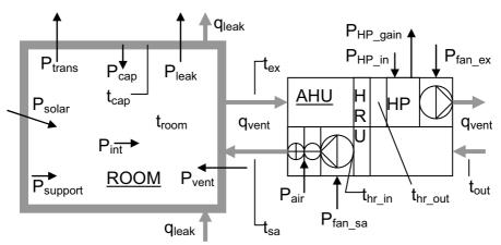
Figure 5.12. The included powers in the power and energy calculation of the LCC model.
