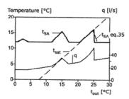
Fig. 11. Optimal supply air temperature  $(t_{SA})$  and supply air flow, q, at different outdoor temperatures  $(t_{out})$ . The load,  $P_{toad}$  increases with an increasing outdoor temperature  $P_{internal} = 400$  W corresponding to 30 W/m<sup>2</sup> floor area, U = 1.67 W/(m<sup>2</sup> °C).  $\eta_1 = 0.5$ ,  $q_{min} = 16$  l/s. The dashed line is the saturation temperature  $(t_{sat})$ .
