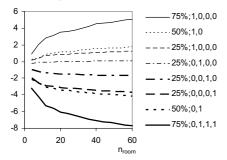
Figure 23. The maximum pressure drop for the average case minus the maximum pressure drop for the correct case for a one-branch supply duct system. The legend gives the occupancy rate followed by the room occupation sequence given by Figure 8.
