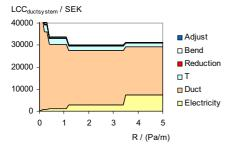
Figure 12. The LCC with its components for a twelve room supply duct system with one branch as a function of a given *R*-value for the first piece of the branch duct. The other pieces of branch ducts had the same size as the first, that means constant size on one level of the duct system.
