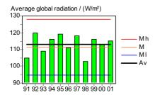
Figure 28. Global horizontal radiation for the readings for each year respectively together with the average from the extreme and normal years of Meteonorm for Lund.
