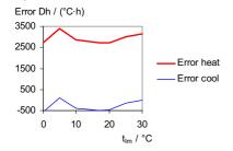
Figure 9. The error between measurements and the Meteonorm normal year in annual degree hours as a function of the limit temperature,  $t_{lm}$ , for Stockholm.
