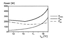
Fig. 14. The power requirement (P<sub>HVAC</sub>) depending on supply air temperature in Case 3 at 23 °C outdoor temperature. Input data according to Fig. 11.
