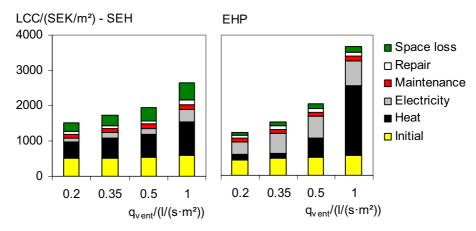
Figure 6.19. The LCC for system 2 and 3 in Table 6.7 as a function of the airflow rate per floor area. SHE means supply and exhaust and EHP, exhaust with exhaust air heat pump.
