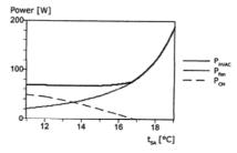
Fig. 13. The power requirement ( $P_{\rm HVAC}$ ) depending on supply air temperature in Case 3 at 16 °C outdoor temperature. Input data according to Fig. 11.
