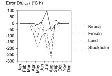
Figure 19. The annual error in degree hours for cooling for each month as the simulated value minus the measured.
