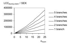
Figure 20. The LCC for the supply duct system as a function of number of rooms per branch and number of branches
