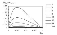
Figure 11. The fan energy use error by using binomial distribution with a zero occupancy airflow rate of 0.33. The legend shows the number of rooms.
