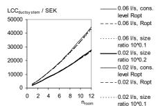
Figure 9. The LCC for a supply duct system similar to Figure 1 but with more rooms on the branch. Here, the approach with size ratio  $10^{0.2}$  is shown.
