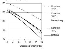
Figure 18. The annual total energy use (without energy for internal heat) when the occupied time is varied symmetrically from 13.00. The calculation was made for Frösön and the office zone was occupied between 08.00 and 18.00.
