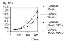
Figure 3. Cost for T-junctions depending on the straight diameter,  $d_A$ , and the connected diameter,  $d_B$ .  $d_A = d_B$  means that the connection duct is of the same size as the main flow duct.  $d_A = d_B \cdot 10^{0.2}$  means that the connection is two standard sizes smaller.
