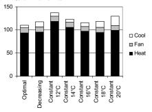
Figure 11. The calculated annual energy use for the simulated office zone in Frösön, central Sweden, per floor area for different supply air temperature control strategies. "Cool" relates to  $P_{cm}$ , "Fan"  $P_{fon}$  and "Heat"  $P_{rad} + P_{hol}$ .
