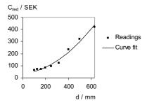
Figure 4. Cost for reductions as a functio of the diameter. The readings follow the standard sizes.
