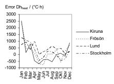
Figure 18. The annual error in degree hours for heating for each month as the simulated value minus the measured.
