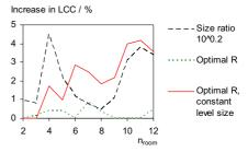
Figure 10. The increase in LCC for a one-branch supply duct system with 125 mm connection ducts compared to the case with all sizes individually set with a size ratio of 10<sup>0.1</sup>.
