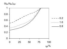
Figure 14. The optimal ratio between supply and exhaust air-flow rate due to an energy use perspective for Malmö. The figures in the legend is  $I_f$  in  $I/(s \cdot m^2)$ .
