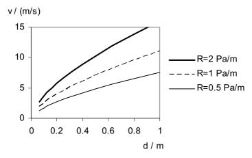
Figure 5.10. The air speed as a function of pressure drop per meter duct and duct diameter according to Equation 5.1 with an air density of 1.2 kg/m³.
