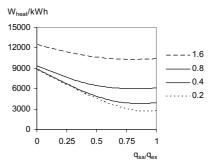
Figure 11. The annual energy use for heating air for Malmö depending on the ratio between supply and exhaust airflow rate. The legend shows  $l_t$  in  $l/(s \cdot m^2)$ .
