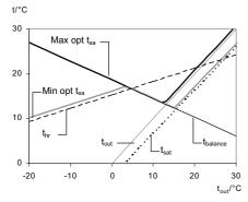
Figure 7. The optimal supply air temperature and the parameters that decides the optimal supply air temperature. Below  $1^{\circ}$ C and above  $12^{\circ}$ C, there is a range of optimal supply air temperatures, between the Max opt  $t_{sa}$  and Min opt  $t_{sa}$ , where the power requirement is the same. Between  $1^{\circ}$ C and  $12^{\circ}$ C, the Max opt  $t_{sa}$  and Min opt  $t_{sa}$  coincide and there is only one optimal supply air temperature.
