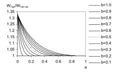
Figure 10. The fan energy use error by using constant average airflow rate for a rectangular distribution with edges in a and b where b > a.
