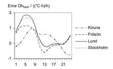
Figure 20. The annual error in degree hours for heating for each hour of the day as the simulated value minus the measured. The sum is divided with 365 to give the error per hour.
