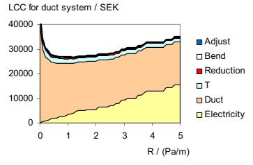
Figure 3.5. The LCC with its components for a twelve room supply duct system with one branch as a function of a given pressure drop per meter, *R*, for each piece of duct. 'Adjust' refers to adjusting dampers, 'Bend' to bends, 'Reduction' to size reductions if needed, 'T' to T-junctions, 'Duct', to ducts and 'Electricity' to fan electricity over 50 years. Adjust, bend and reduction is negligible in the graph.
