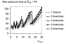
Figure 19. The maximum duct pressure drop in the case shown in Figure 17 with optimal *R* when *R* was set for the first duct piece in the branch and main ducts respectively for a supply duct system. The connection ducts were 125 mm in diameter.
