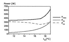
Fig. 15. The power requirement (P<sub>HVAC</sub>) depending on supply air temperature in Case 4 at 26 °C outdoor temperature. Input data according to Fig. 11.
