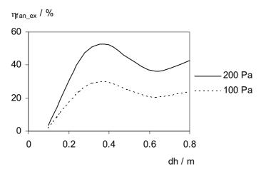
Figure 5.13. The outer fan efficiency for exhaust fans at L=3.4 at the outer pressure difference of 200 Pa and 100 Pa respectively.
