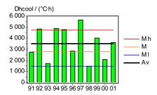
Figure 14. Annual degree hours for cooling for the readings for each year respectively together with the average from the extreme and normal years of Meteonorm for Lund.
