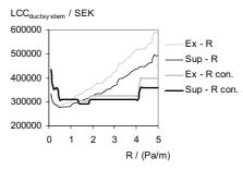
Figure 14. The LCC for a four branch, twelve room per branch duct system as a function of *R* for supply (Sup) and exhaust (Ex) systems. 'R' means that every piece in the branch used *R* as max value. 'R con.' means that the branch size was held constant.
