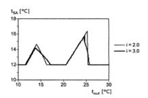
Fig. 16. Optimal supply air temperature with different exponents (i) in Eq. (5).  $P_{\rm internal}=400\,{\rm W}$  (corresponding to  $30\,{\rm W/m^2}$  floor area) and U=0.
