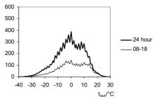
Figure 5. The annual temperature frequency for Kiruna for the period 1991-2001. The lower curve shows the daytime hours only.
