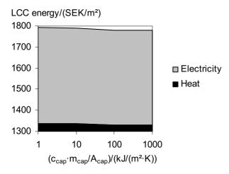
Figure 6.8. The energy part of the LCC as a function of the average thermal mass of the interior for the default CAV system.
