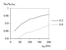
Figure 13. The optimal ratio between supply and exhaust air-flow rate due to an energy use perspective for Malmö. The figures in the legend is  $I_f$  in  $I/(s \cdot m^2)$ .
