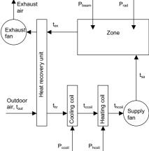
Figure 1. The studied HVAC system and the office cell.
