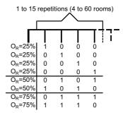
Figure 8. Different flow distributions compared to the average airflow rate set for all rooms. '1' means  $0.02 \text{ m}^3/\text{s}$  while '0' means zero airflow rate.  $O_R$  is the occupancy rate.
