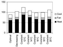
Figure 10. The calculated annual energy use for the simulated office zone in Lund, South Sweden, per floor area for different supply air temperature control strategies. "Cool" relates to  $P_{\it cmh}$  "Fan"  $P_{\it fom}$  and "Heat"  $P_{\it rad}+P_{\it boil}$ .
