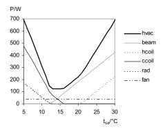
Figure 8. The different power used by the HVAC system in the example for 15°C outdoor temperature. To the right,  $P_{heatt}$  and  $P_{heatt}$  is positive and  $P_{ccoll}$  and  $P_{rad}$  is zero. At 12°C, condensation starts in the supply air with a change in the derivative of the  $P_{ccoll}$ .
