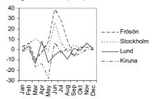
Figure 32. The error in monthly average global radiation as the simulated value minus the measured.
