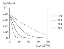
Figure 8. The annual average leakage as a ratio of the leakage factor,  $I_6$  for Kiruna.
