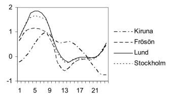
Figure 3.7. The annual error in degree hours split into each hour of the day as the simulated value minus the measured. The value at 17.00 refers to the hour before, which means 16.00 to 17.00. The summed error is divided with 365 to give the error per hour.
