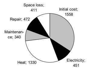
Figure 6.1. The different components of the LCC in SEK/m<sup>2</sup> excluding VAT for the example in Section 6.1. The area in the denominator is  $A_{BTA}$
