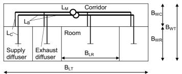
Figure 5.2. The assumed typical single sided premises seen from above. The assumed lengths of the duct pieces pointed out,  $L_M$ , which is perpendicular to the paper in the sketch,  $L_b$  and  $L_C$ , are given in Table 5.3.
