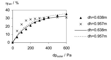
Figure 5.14. Measured and modelled outer fan efficiencies for larger air handling units with exhaust and supply fan. The airflow rate is  $1 \text{ m}^3/\text{s}$ .
