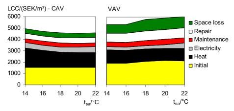
Figure 6.4. The LCC as a function of the supply air temperature for the systems 1 and 15 in Table 6.2.
