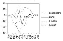
Figure 37. The error in monthly average global radiation as the simulated value minus the measured.
