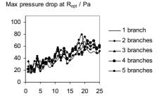
Figure 18. The maxium pressure drop in the case shown in Figure 16 with optimal R when R was set for every duct piece in the branch and main ducts. The connection ducts were 125 mm in diameter.
