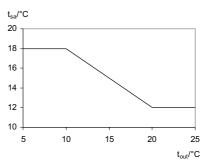
Figure 2. The supply air temperature as function of outdoor temperature for the denoted "decreasing strategy".
