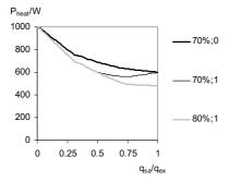
Figure 10. The total power for heating the air at default conditions. The legend gives  $\eta_0$  and  $\alpha$  respectively.
