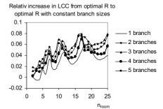
Figure 17. The relative increase from the duct system based on  $R_{opt}$  for each duct piece individually and the case when the size has been constant for each branch and the main duct respectively for a supply duct system
