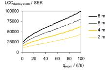
Figure 22. The duct system optimal LCC for a one branch, twelve rooms supply duct system depending on the air flow rate for each room. The optimization method was to set maximum *R* for every duct piece in the branch and main duct. The connection ducts were 125 mm. The length between each room, was varied between 2 and 8 meter.
