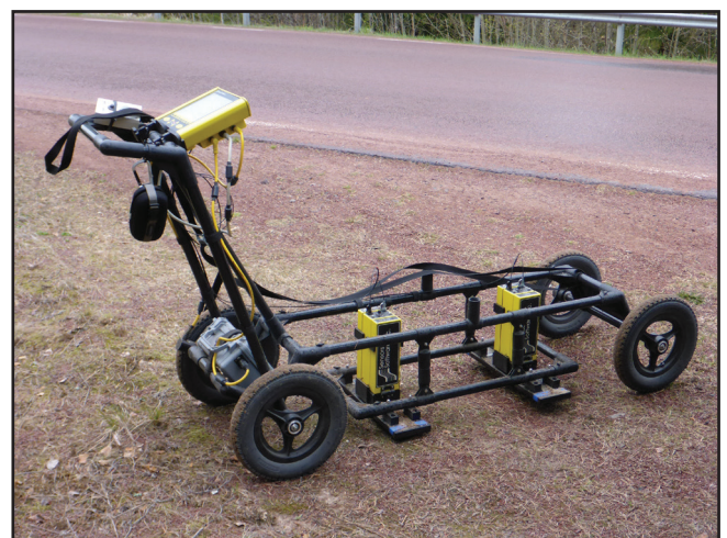
Fig. 12. Image of the GPR used during field work. Image courtesy of Helena Alexanderson.
