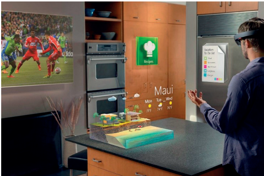
Figure 6. Example of an AR application superimposing virtual objects on the real world through the Microsoft HoloLens. Image adapted from Coldewey (2015).
