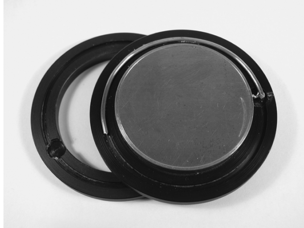
Figure 5.3: The physical implementation of our pacemaker model, here with the circumference antenna.
