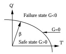
Figure 3. Reliability index b in a two dimensional standardised space with the basic variables Q and T. G=0 indicates the limit state function =0.
