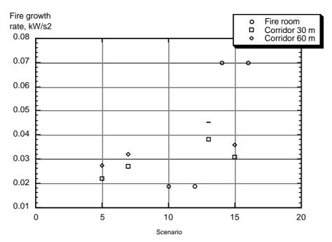
Figure 11. Design value for the fire growth rate derived with the FOSM method.
