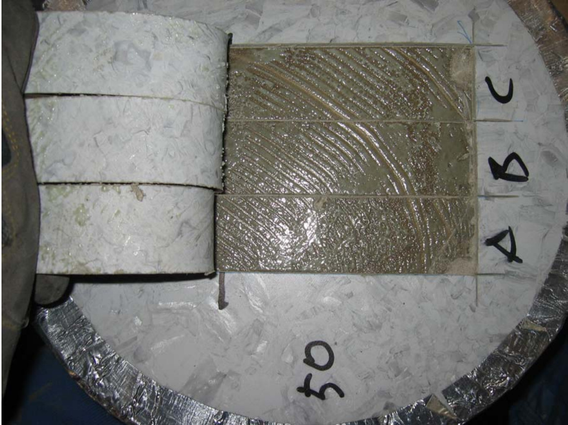
Appendix 5.50 – Fracture view at peel test of specimen no 50
