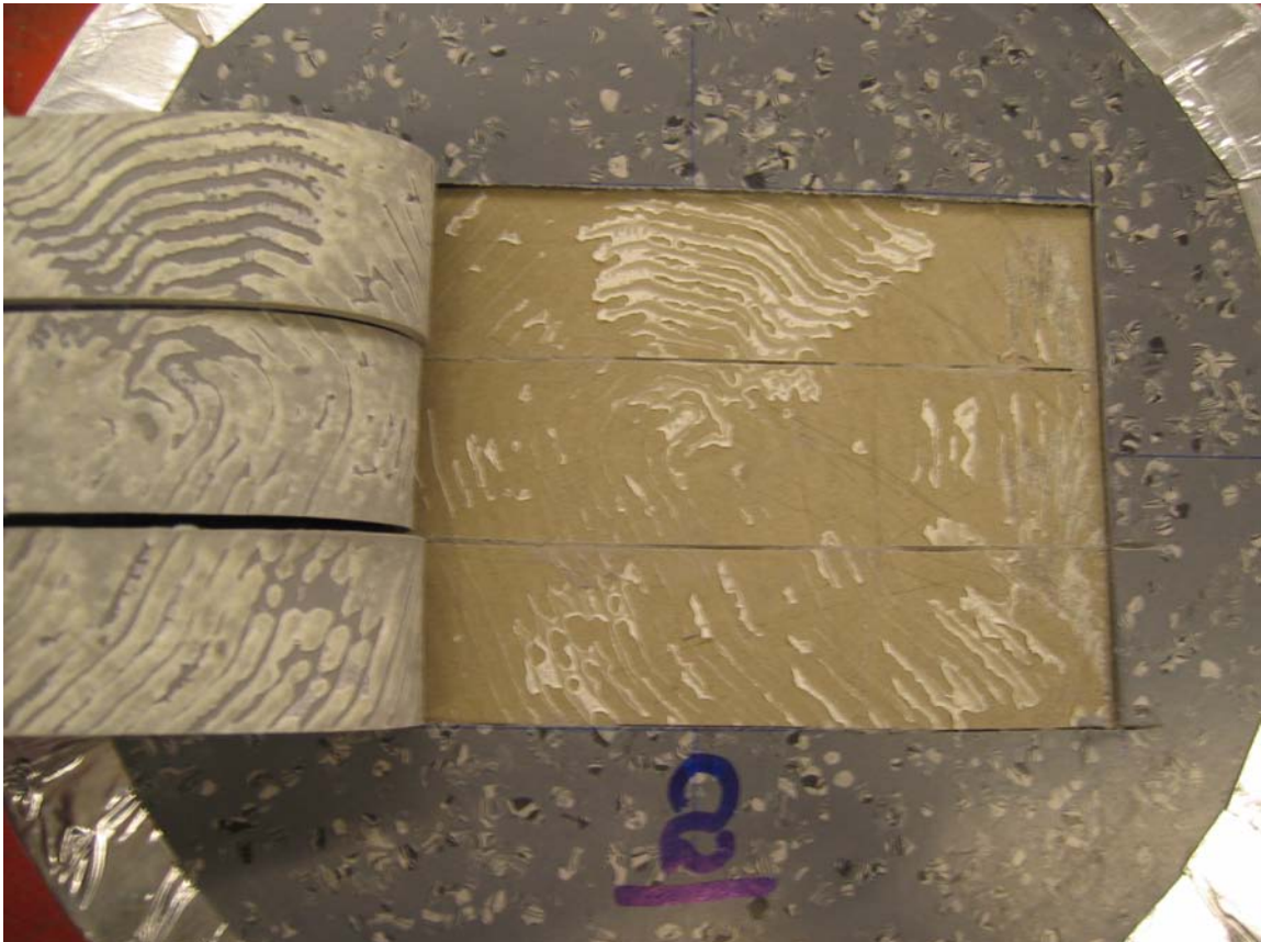
Appendix 5.2 – Fracture view at peel test of specimen no 2
