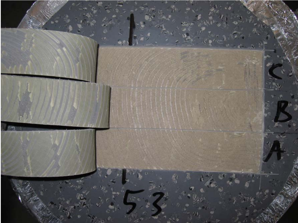
Appendix 5.54 – Fracture view at peel test of specimen no 54
