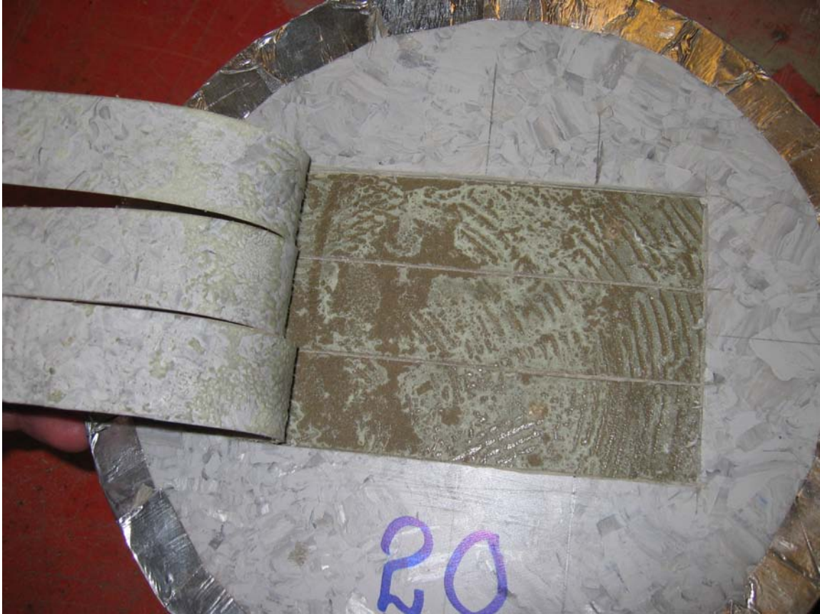
Appendix 5.20 – Fracture view at peel test of specimen no 20
