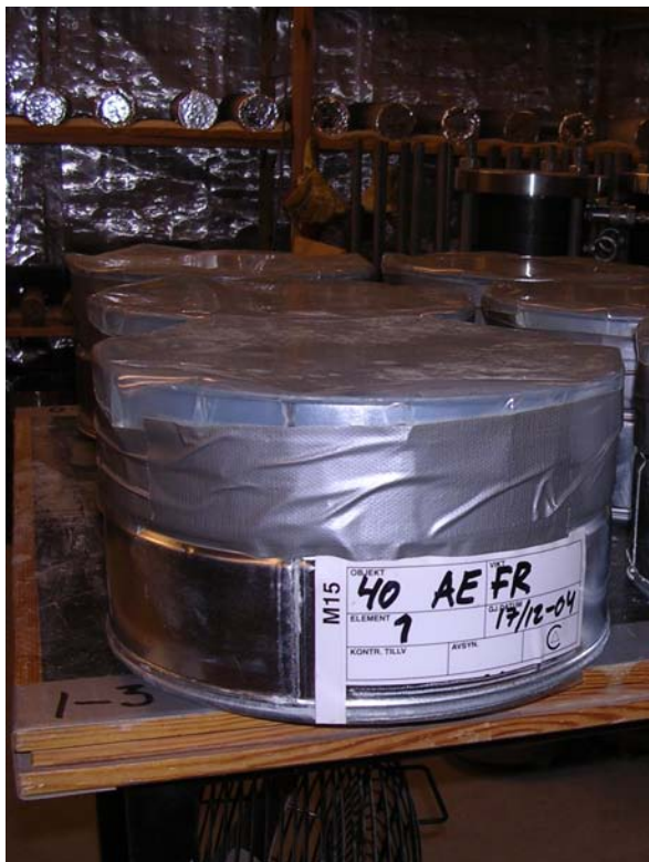
Figure 3.1 - Concrete casting within an Ø250 x 140 mm steel ventilation tube with a socket tightened with a rubber sleeve.
