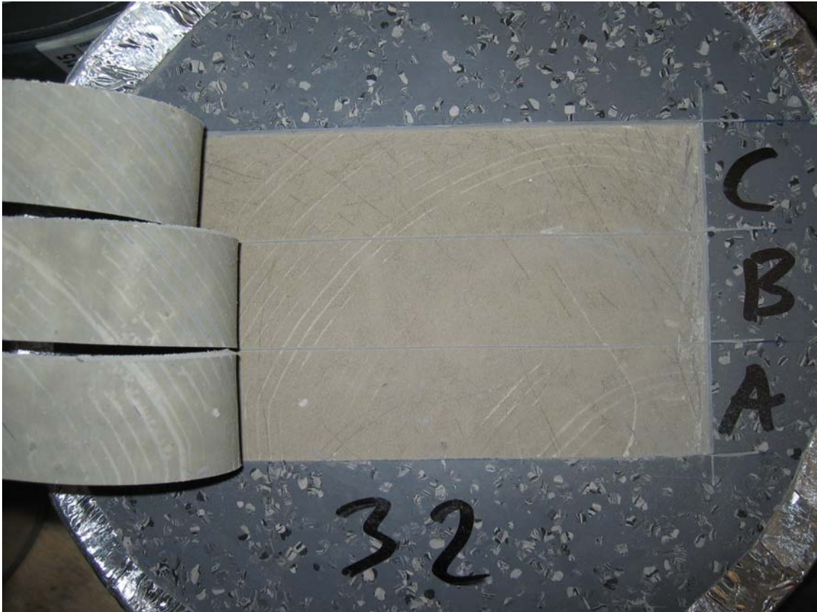
Appendix 5.32 – Fracture view at peel test of specimen no 32
