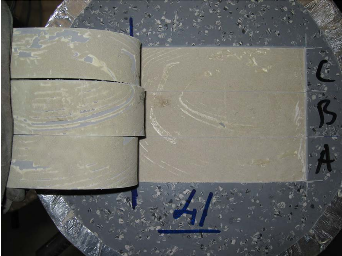
Appendix 5.42 – Fracture view at peel test of specimen no 42
