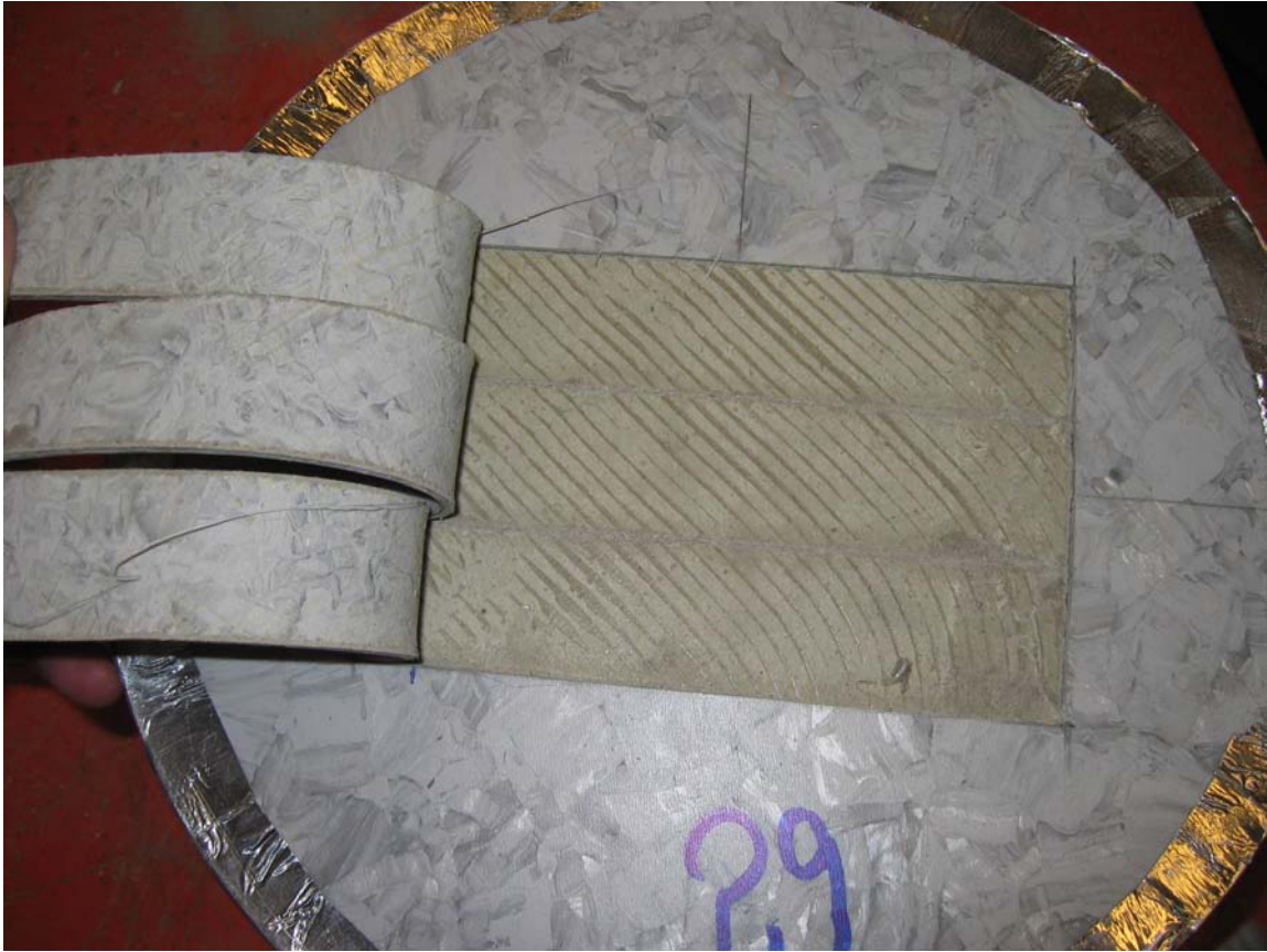
Appendix 5.30 – Fracture view at peel test of specimen no 30
