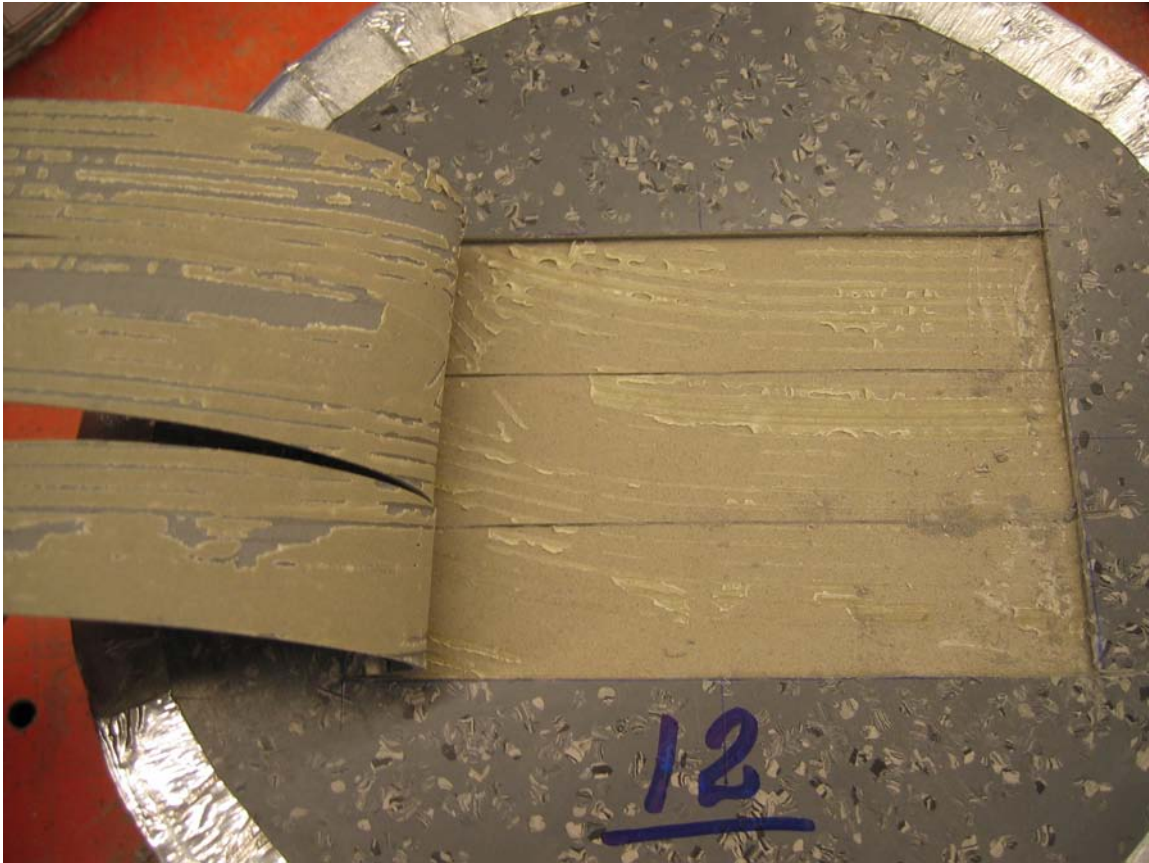
Appendix 5.12 – Fracture view at peel test of specimen no 12
