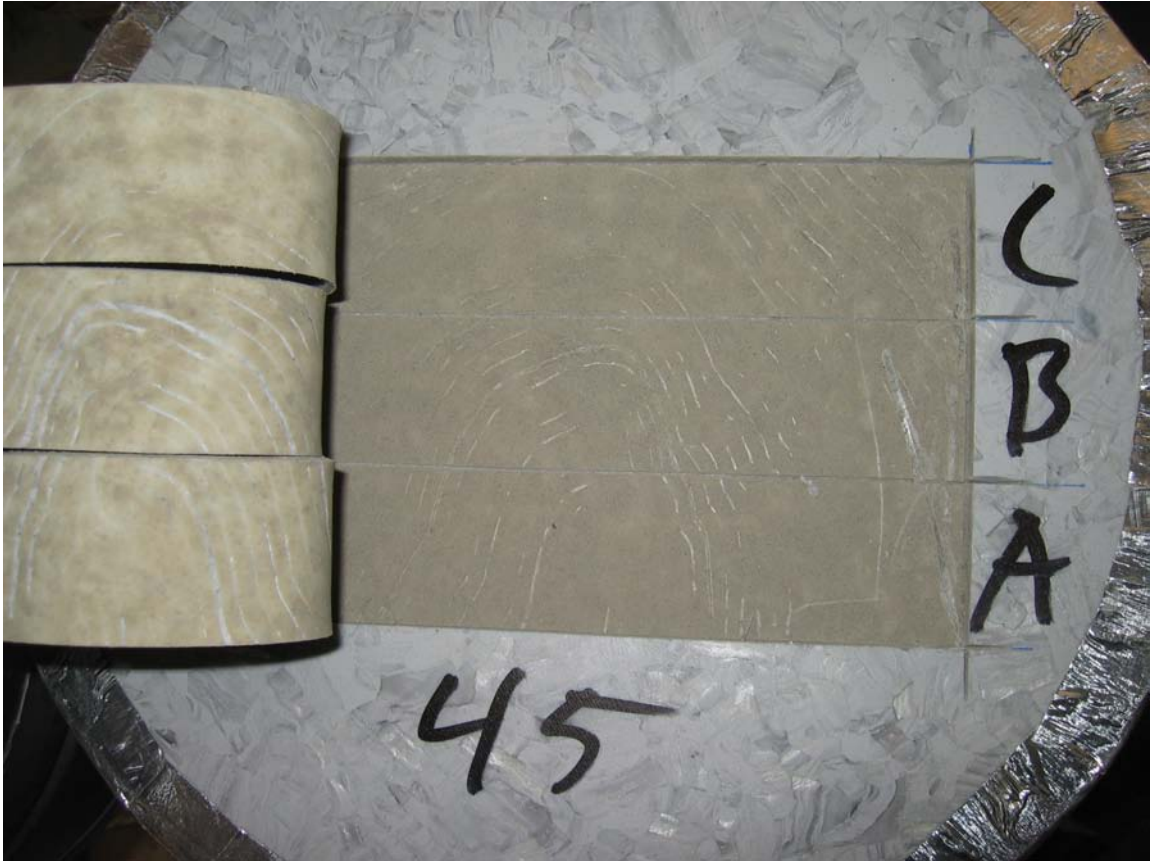
Appendix 5.46 – Fracture view at peel test of specimen no 46
