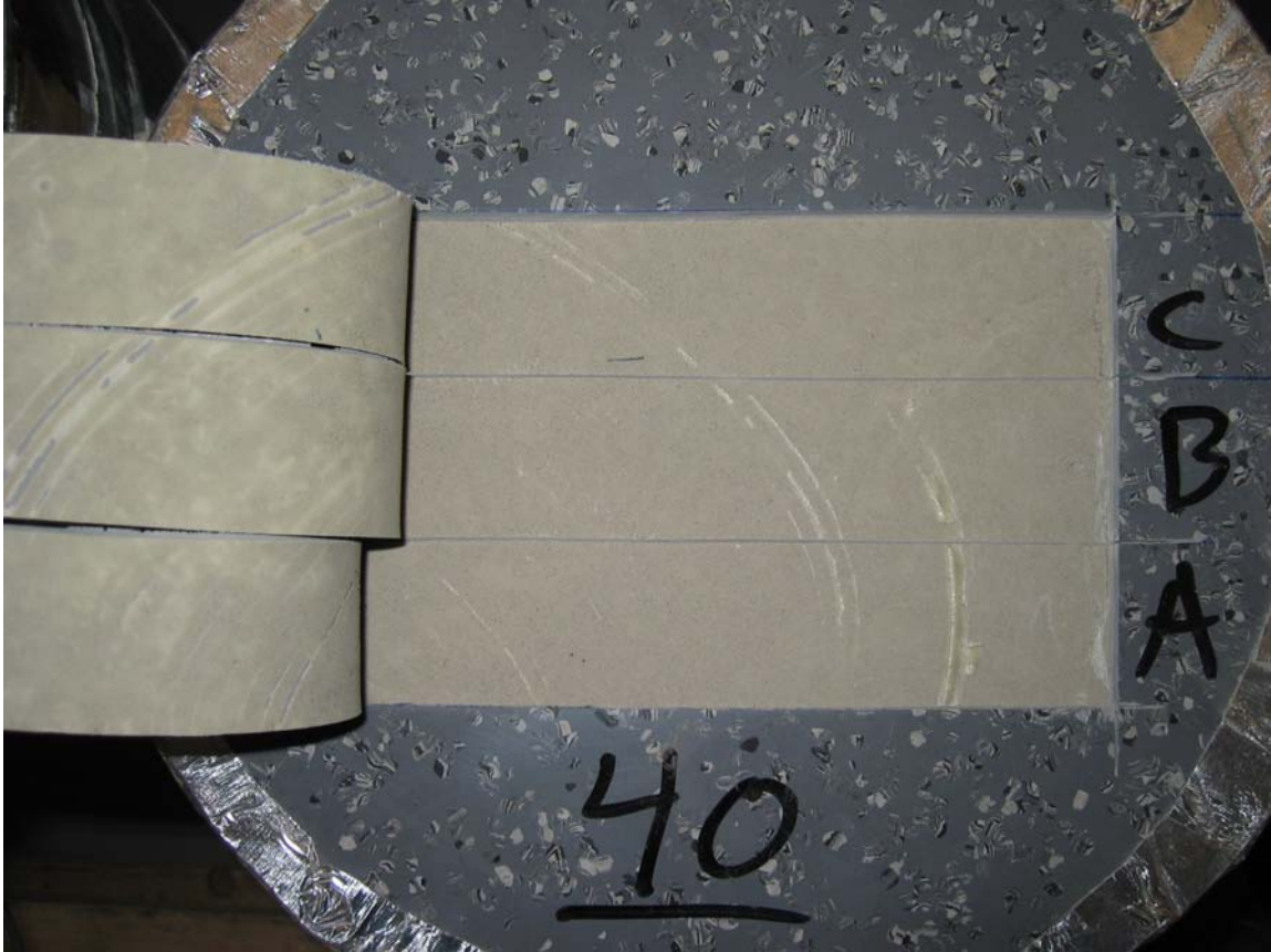
Appendix 5.40 – Fracture view at peel test of specimen no 40
