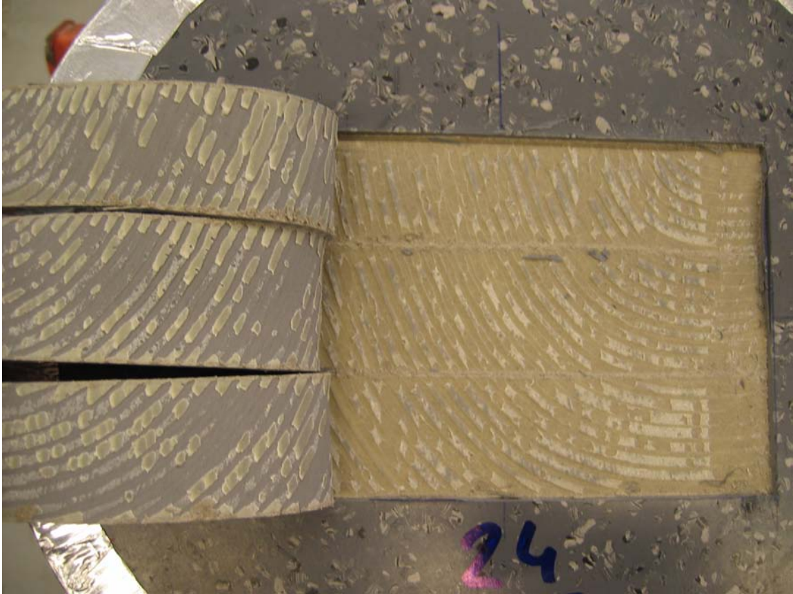
Appendix 5.24 – Fracture view at peel test of specimen no 24
