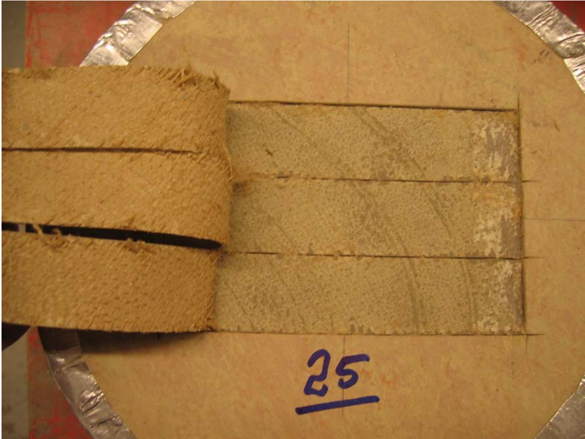
Appendix 5.26 – Fracture view at peel test of specimen no 26
