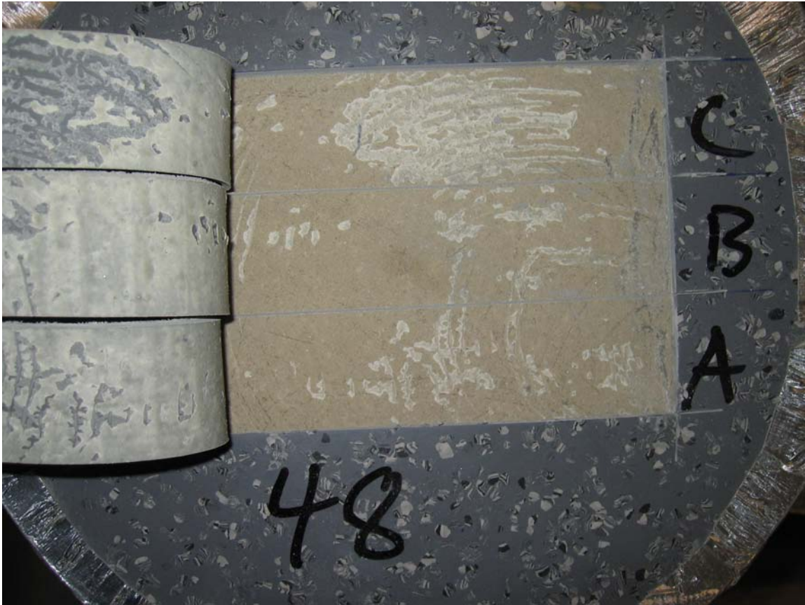
Appendix 5.48 – Fracture view at peel test of specimen no 48
