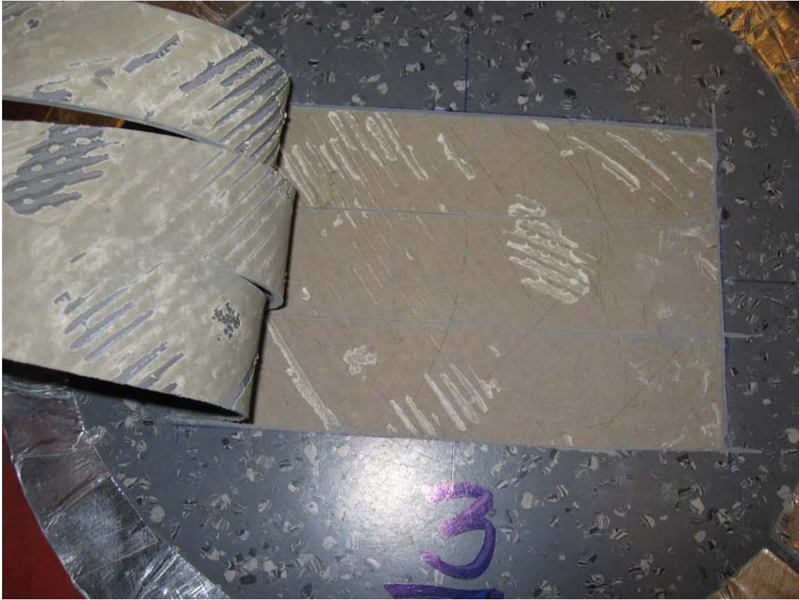
Appendix 5.4 – Fracture view at peel test of specimen no 4
