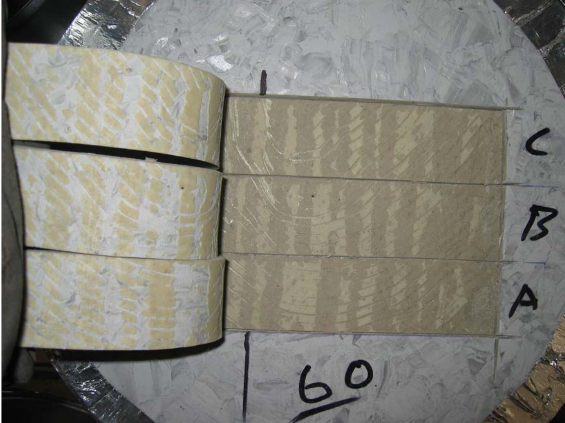
Appendix 5.60 – Fracture view at peel test of specimen no 60
