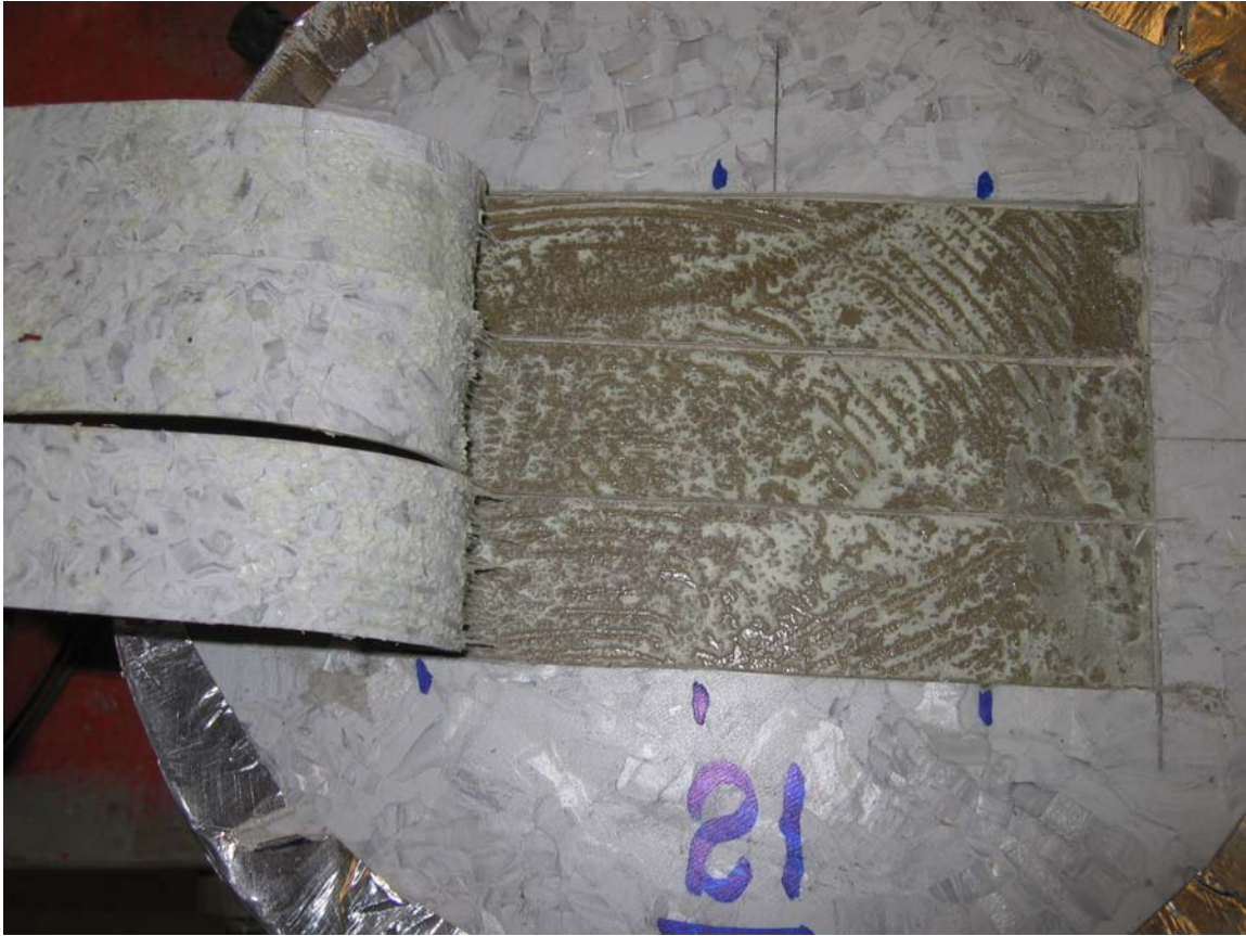
Appendix 5.22 – Fracture view at peel test of specimen no 22
