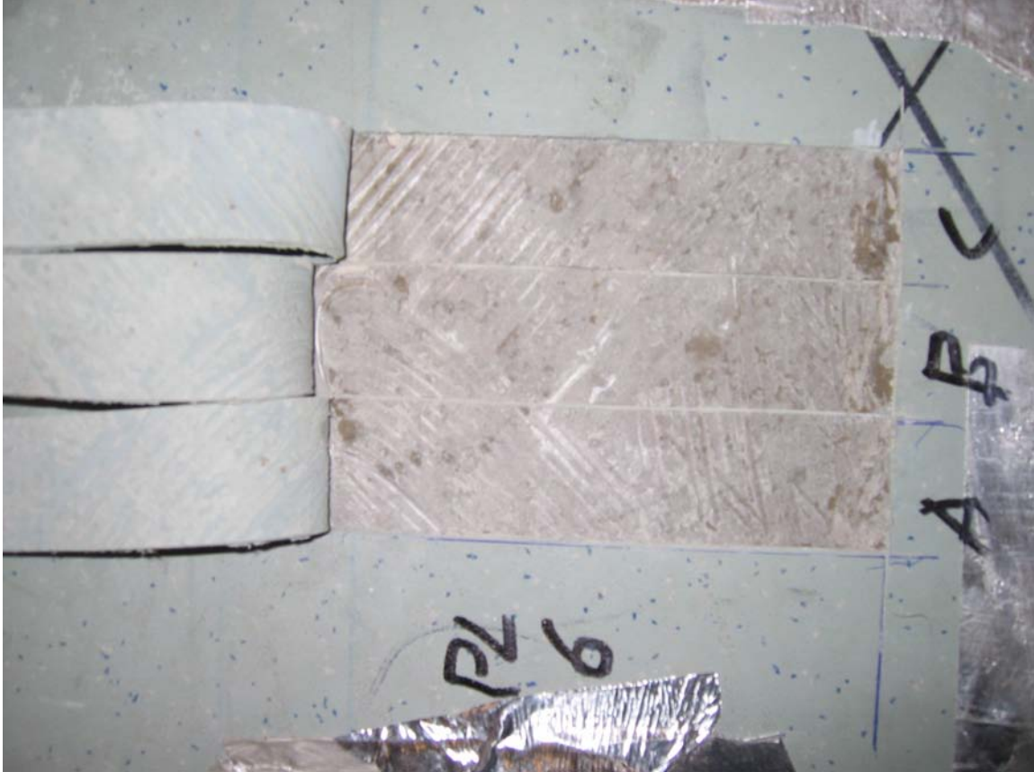
Appendix 5.66 – Fracture view at peel test of specimen no 60BEFR6h
