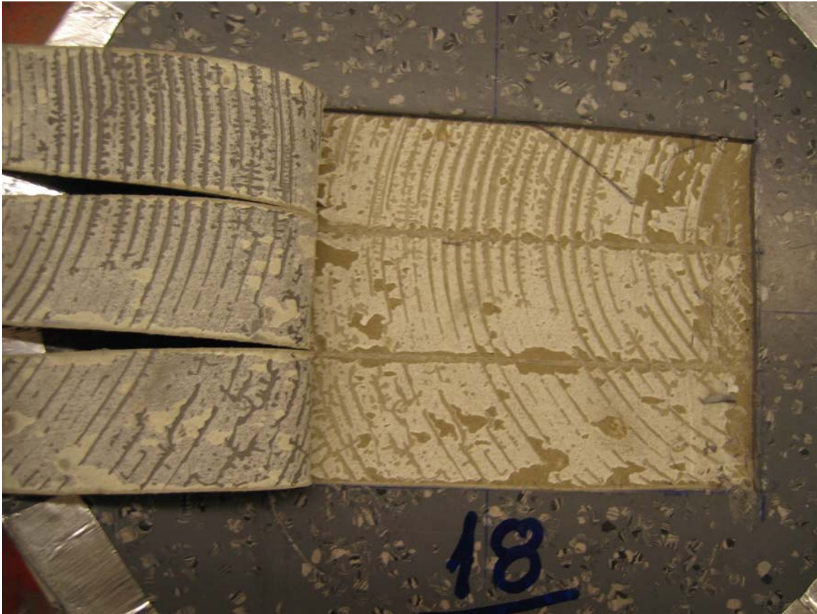
Appendix 5.18 – Fracture view at peel test of specimen no 18
