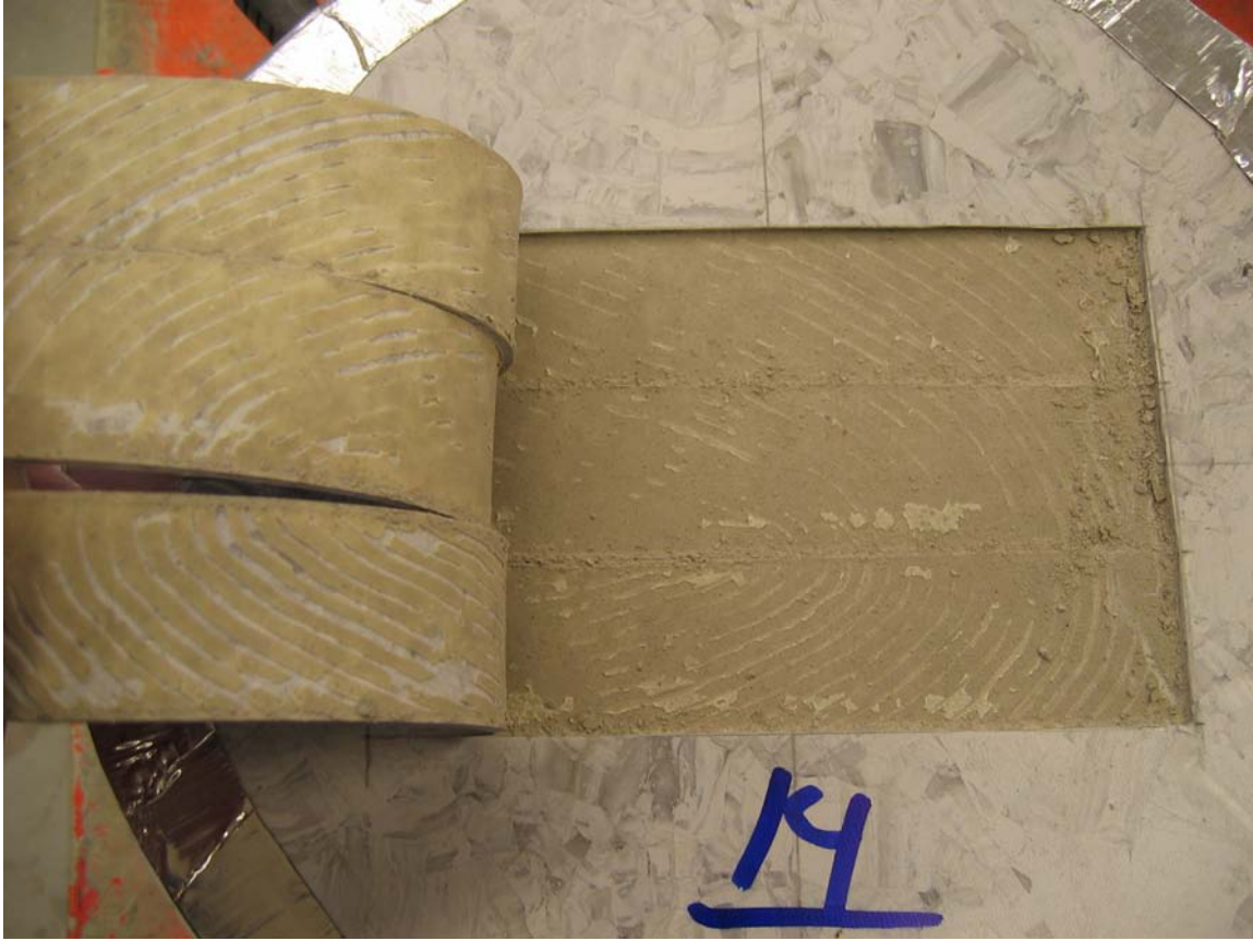
Appendix 5.14 – Fracture view at peel test of specimen no 14
