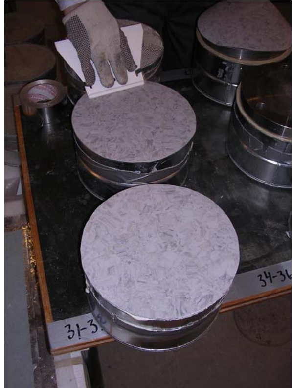
Figure 3.4 - Flooring application tightened at specimen edge with aluminium tape.
