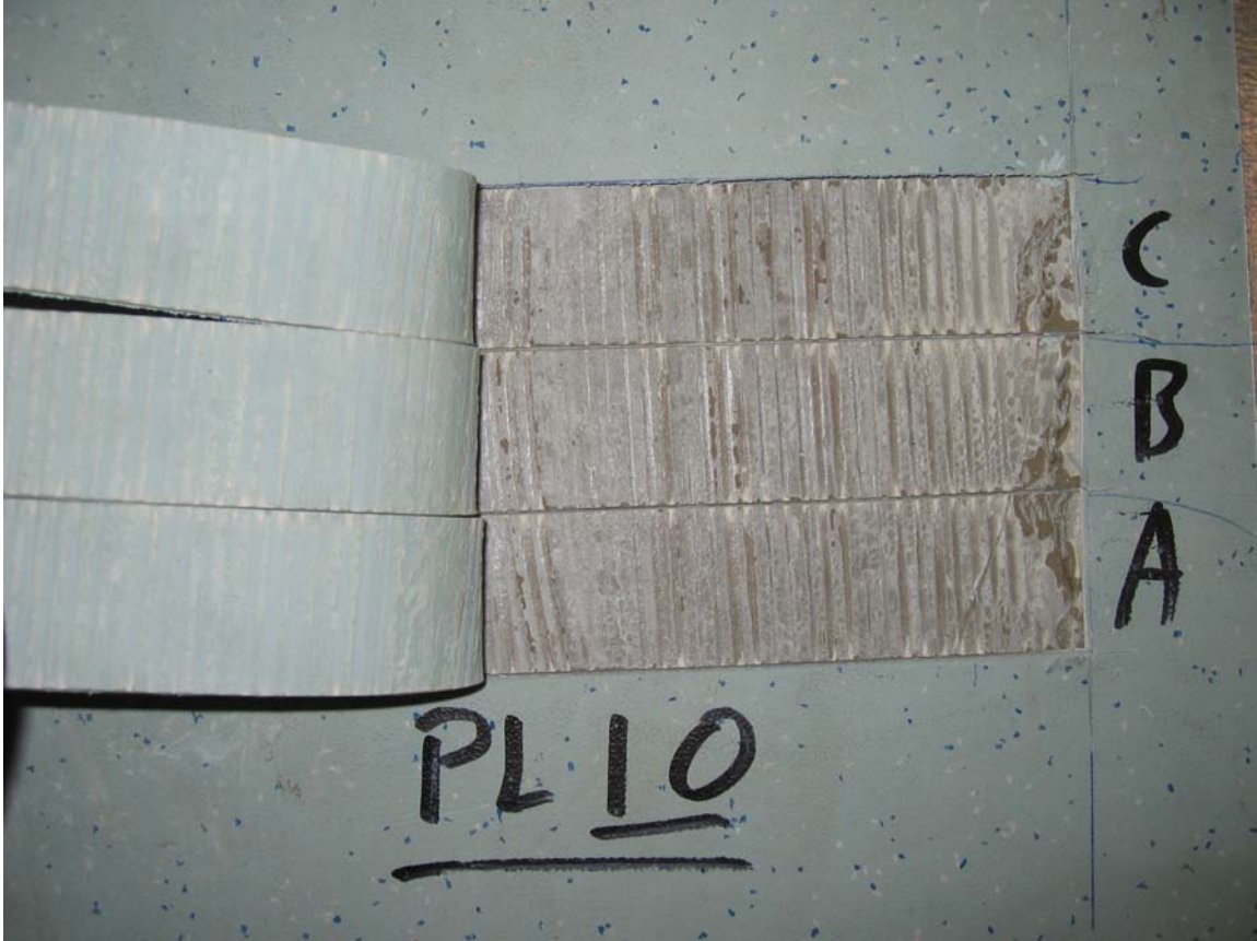
Appendix 5.64 – Fracture view at peel test of specimen no 40BEFR10
