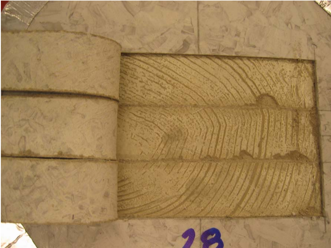
Appendix 5.28 – Fracture view at peel test of specimen no 28
