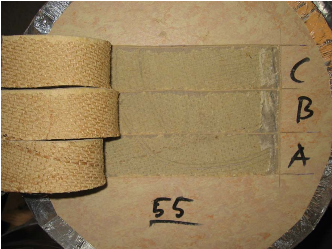
Appendix 5.56 – Fracture view at peel test of specimen no 56
