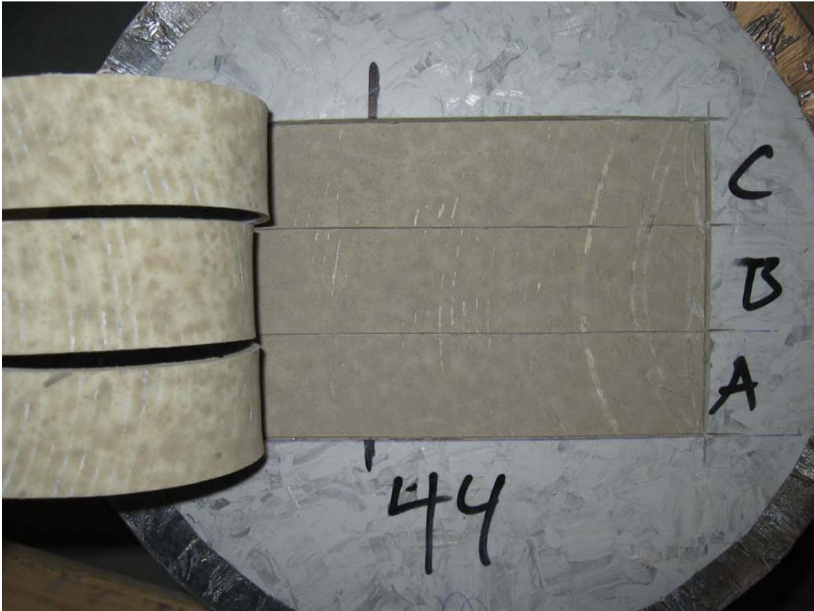
Appendix 5.44 – Fracture view at peel test of specimen no 44
