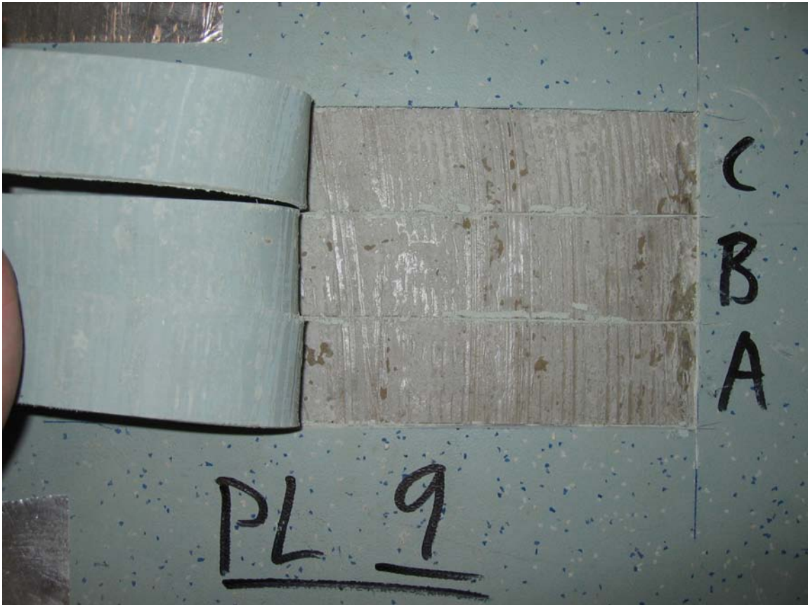
Appendix 5.64 – Fracture view at peel test of specimen no 40BEFR10
