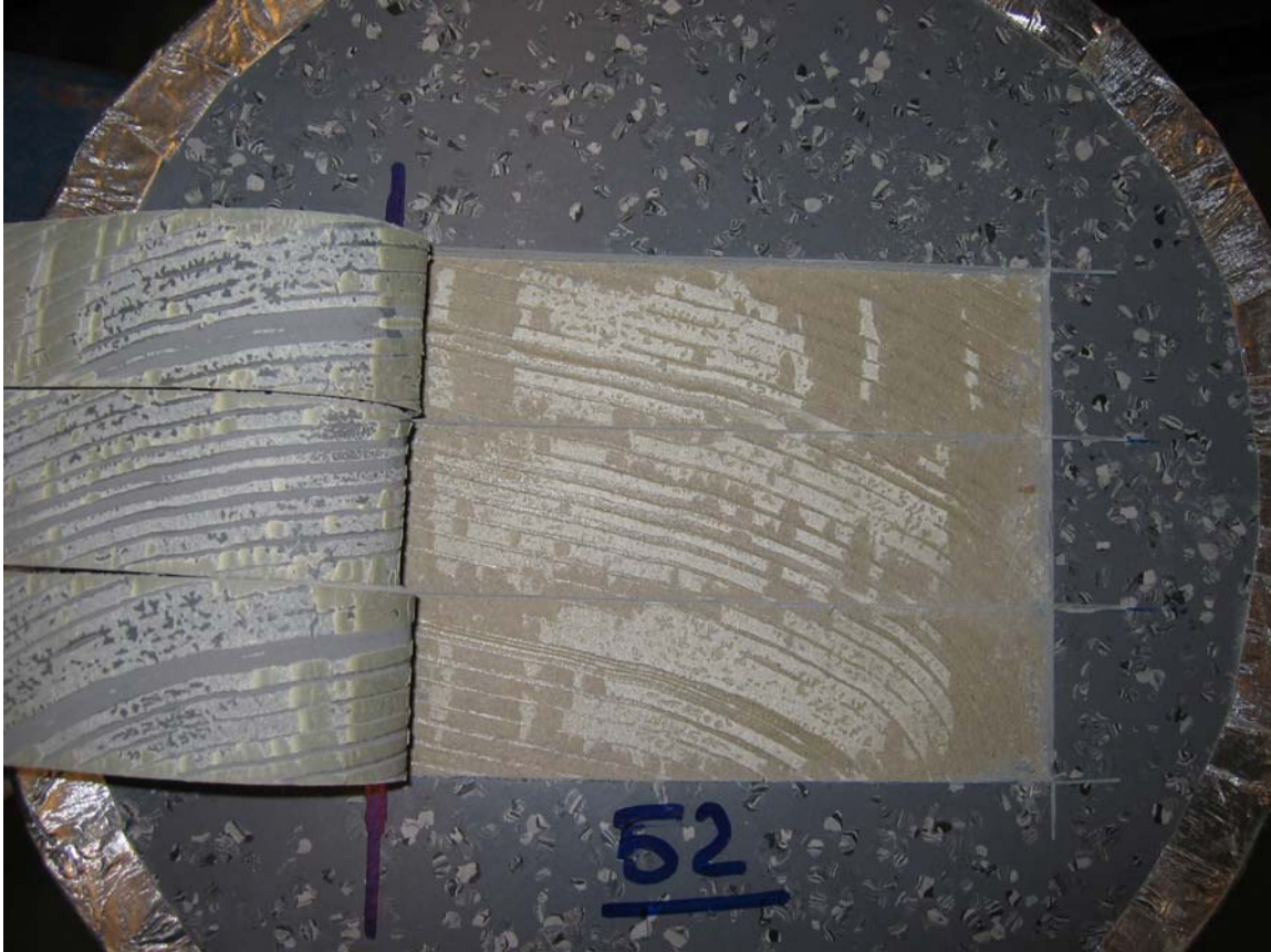
Appendix 5.52 – Fracture view at peel test of specimen no 52
