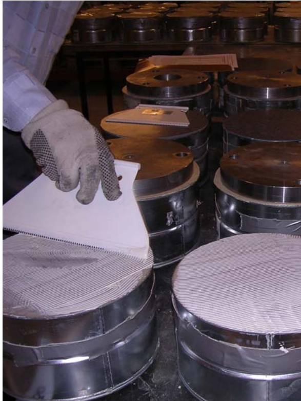
Figure 3.3 - Adhesive application, 3.5 or 4 m 2 /kg, 15 or 25 min drying time at 20 °C and RH = 60%.
