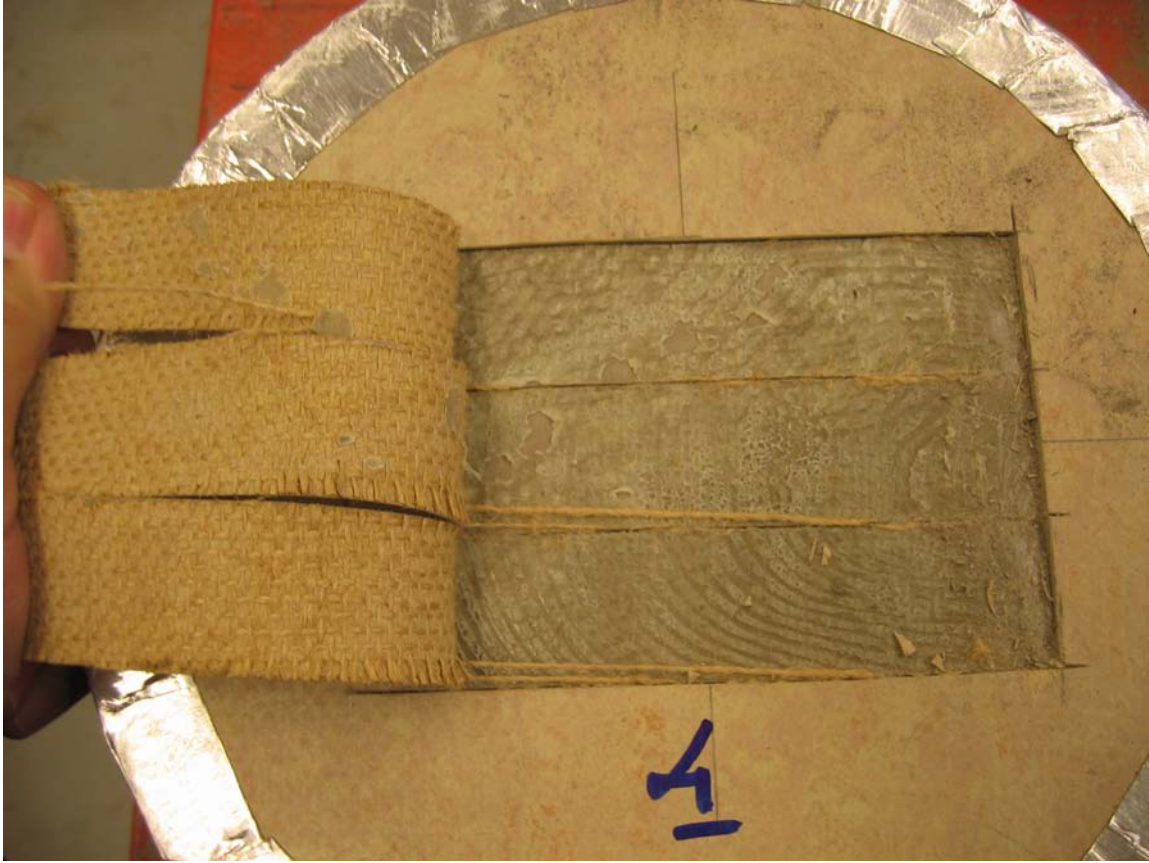
Appendix 5.4 – Fracture view at peel test of specimen no 4
