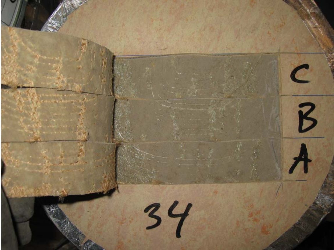
Appendix 5.34 – Fracture view at peel test of specimen no 34
