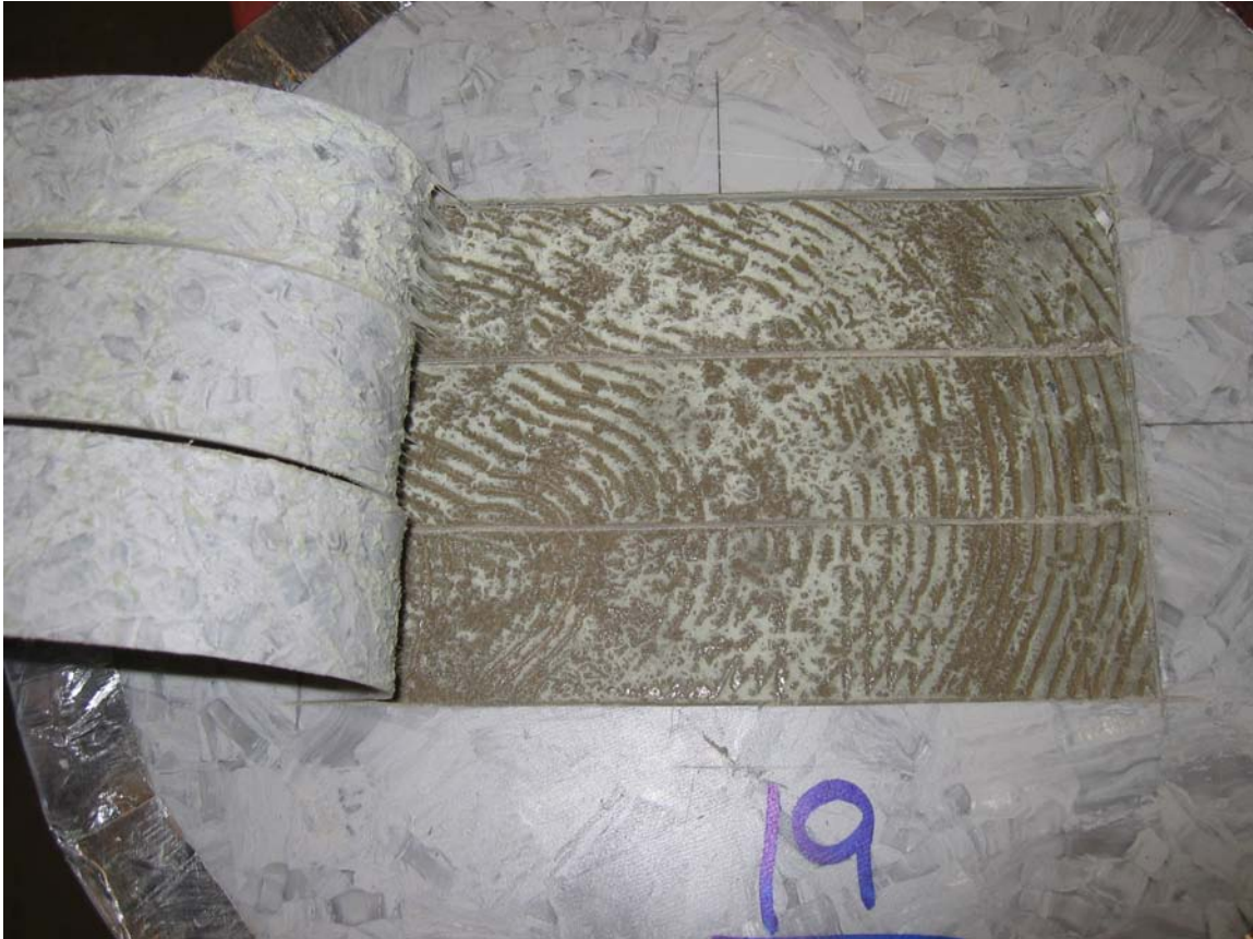
Appendix 5.20 – Fracture view at peel test of specimen no 20
