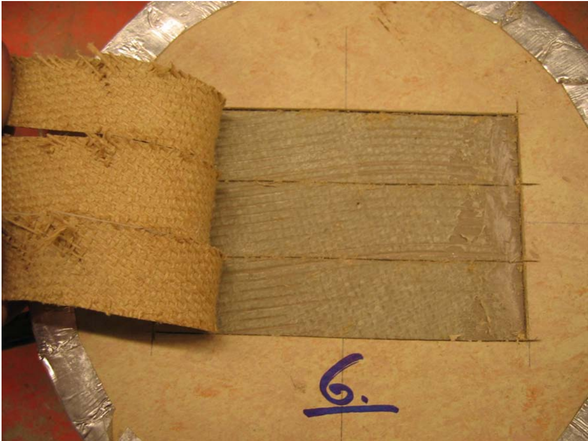
Appendix 5.6 – Fracture view at peel test of specimen no 6
