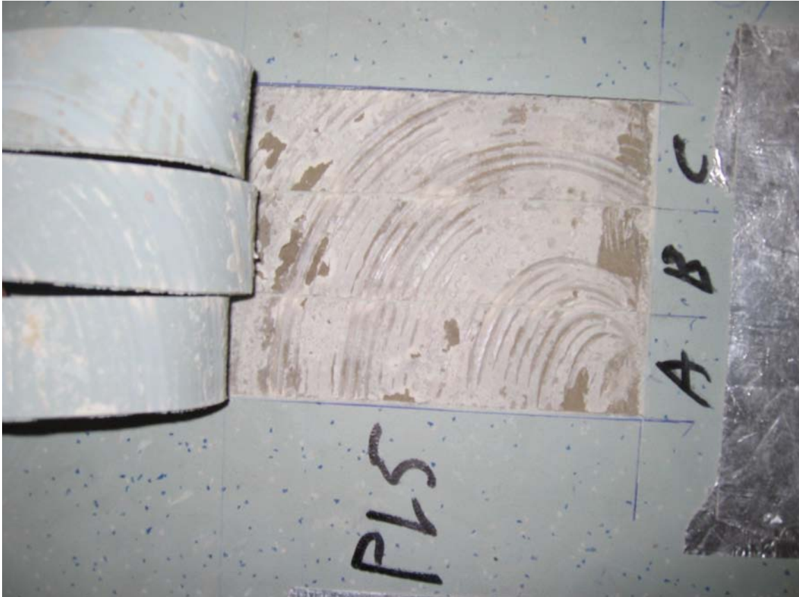
Appendix 5.66 – Fracture view at peel test of specimen no 60BEFR6h
