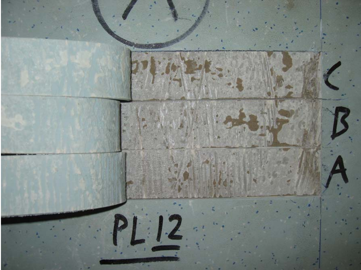
Appendix 5.68 – Fracture view at peel test of specimen no 60BEFR12
