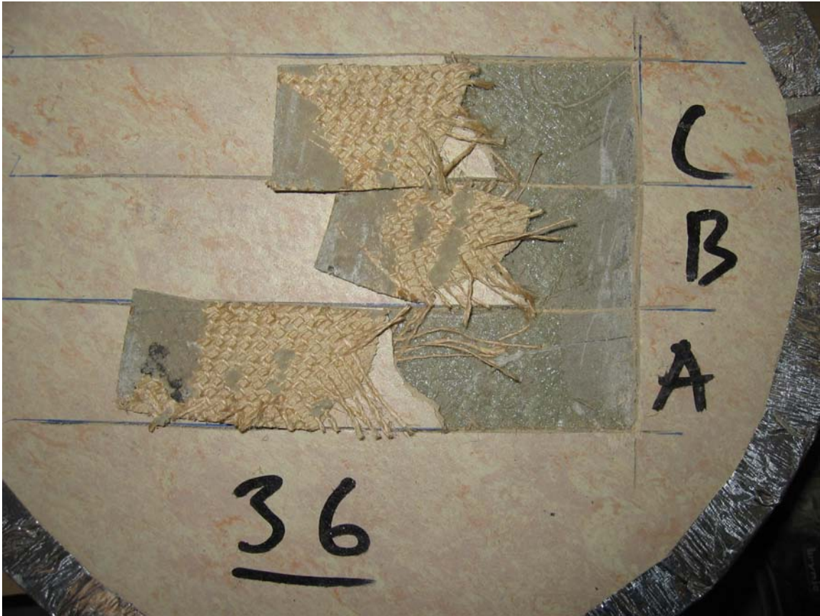
Appendix 5.36 – Fracture view at peel test of specimen no 36
