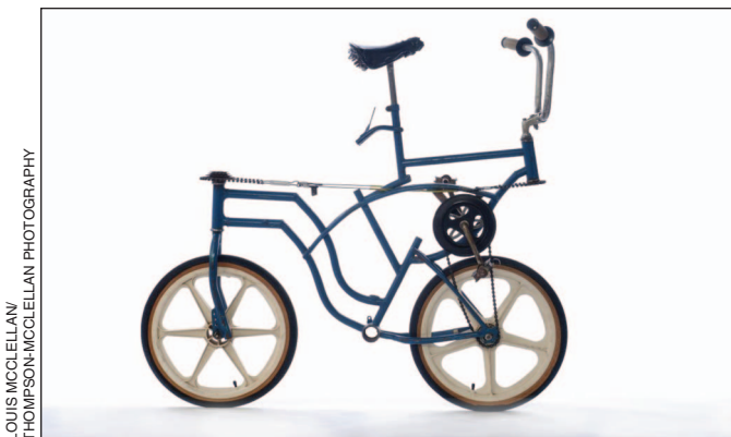
Figure 19. Klein’s rideable rear-steered bicycle. This bicycle is rideable because the rider has a high center of gravity and because the vertical projection of the center of mass of the rider is close to the contact point of the driving wheel with the ground.
