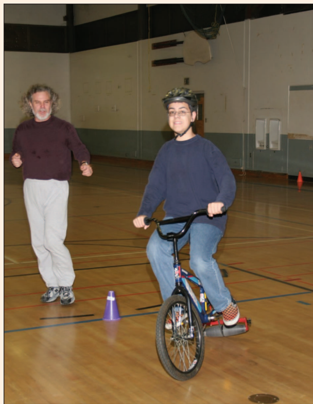
Figure 23. A child on an adapted bicycle with a crowned roller on the rear wheel and a regular front wheel. The child is participating in steering by gently turning the handlebars into the direction of tilt.
