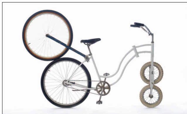
Figure 12. The UIUC naive bicycle with precession canceling. This bicycle is used to demonstrate that a bicycle is rideable even when there are no gyroscopic effects. The bicycle is similar to the bicycle in Figure 11 but has a vertical front fork ( \lambda = 90^\circ ) and zero trail ( c = 0 , see Figure 1), which means that the front fork does not turn when the bicycle is tilted.
