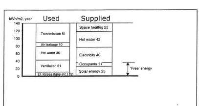
Figure 5. Example of energy balance. Multi-family residential building in Stockholm, built 1985.[5]
