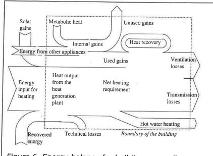
Figure 6. Energy balance for buildings according to CEN. [6] (Metabolic = from occupants)
