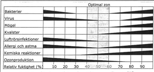
Figure 7. Optimal indoor relative humidity according to [7]. Increased height on triangles => increased risk.
