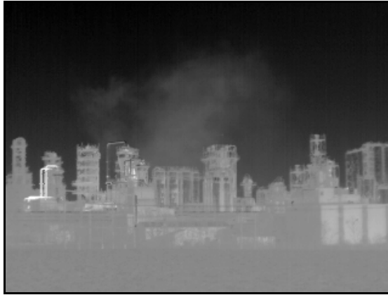
Fig. 5. Ethene gas cloud covering part of the industry five minutes after the high-pressure reactor safety valve release of 1 – 2 tons of ethene into the atmosphere.
