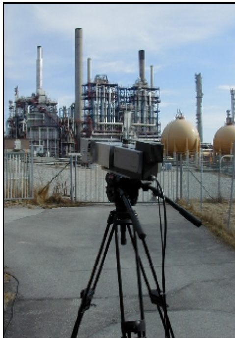
Fig. 1. The gas-correlation infrared camera system in front of a cracker plant.
