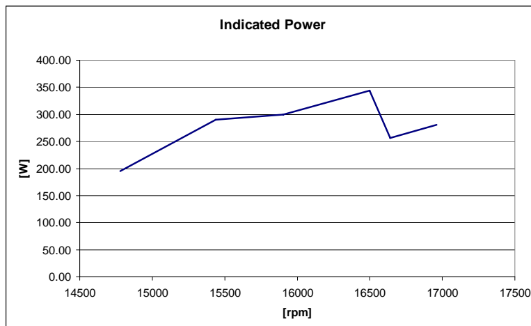
Figure A1-2: The indicated power measured between 14500 and 17500 [rpm].
