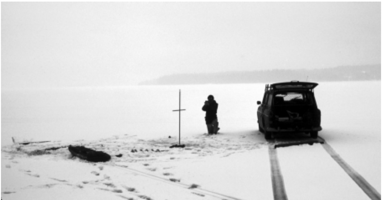
Fig. 1. Photo from the field work at Lake Bolmen during winter. The orientation of the corer is measured, relative to magnetic north.
