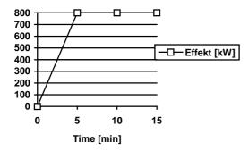
In the detection and activation calculations, the fire is assumed to be "medium", which corresponds to a fire growth factor of  $0.012 \ kW/s^2$ .
