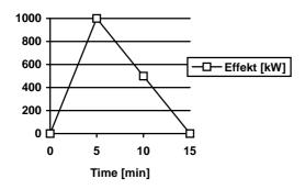
In the detection and activation calculations, the fire is assumed to be "fast" Fire K4
