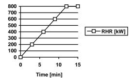
Figure 6.1. Design fire in assembly room
