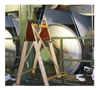
**Figure 5.1** The temperature measuring equipment mounted at cylinder 33.
