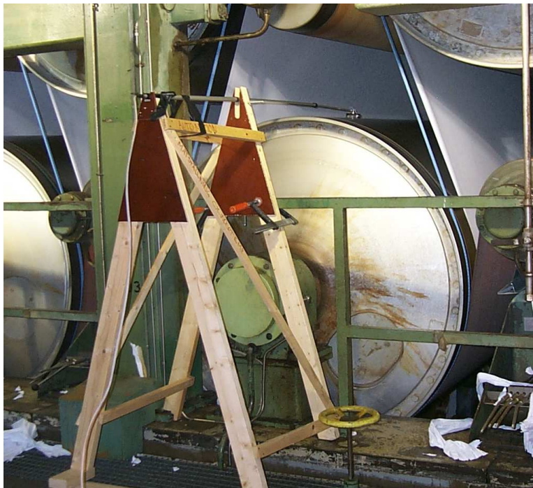
Figure 5.1 The temperature measuring equipment mounted at cylinder 33.
