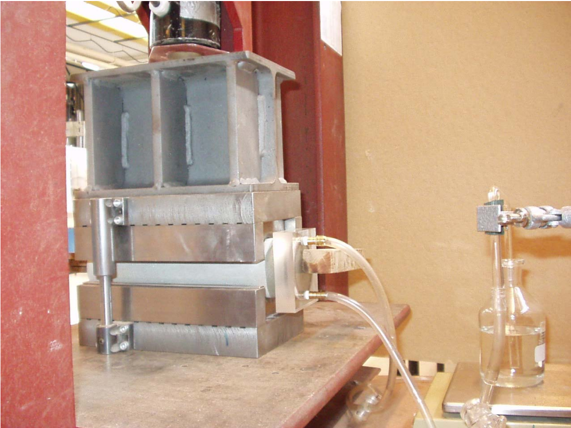
Figure 4.2a Cutting equipment with the stabilization beam attached on top. The complete equipment setup is placed in a rig equipped with a hydraulic jack. Tests were performed on Gotland sandstone prepared as a cylindrical specimen.
