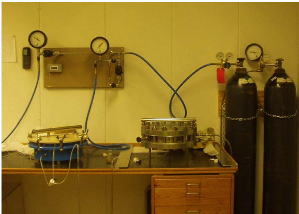
Figure 2.8 Two different pressure plate extractors operating at maximum pressures of 1.5 MPa and 10 MPa, connected to gas cylinders.
