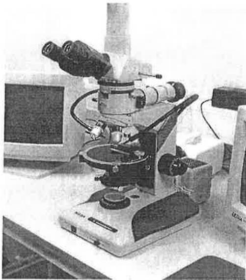
Figure 3: *Microscopic measurements with the LABEYE equipment. Several pictures is analysed for each specimen to obtain the size of circles (bubbles) which are registered in different class intervall by the computer.*
