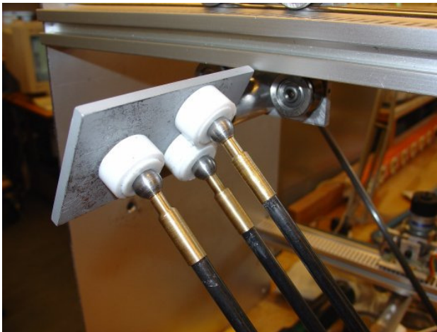
Figure 3.2 Magnetic spherical joints for easy reconfiguration of arm links for the table model of the Gantry-Tau parallel kinematic robot.
