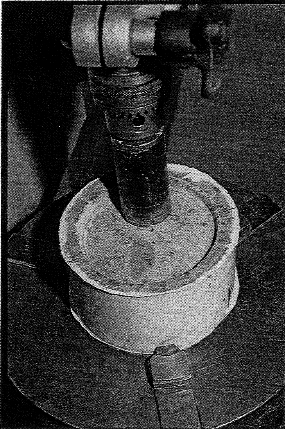
Photo 21. Equipment used for profile grinding, e.g. the successive abrasion of concrete from the exposed surface and inwards. The concrete core is fixed in a lathe while 0.7-2 mm thick layers of concrete are abraded by a rotating diamond tool.
