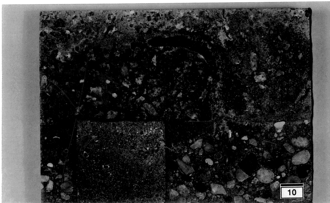
Photo 6. Microstructure and chloride penetration in concrete corrosion cell. Slag cement w/c ratio 0.40, after 8 months exposed to cycles of 2 hours wetting in a 16 % NaCl solution and 166 hours drying in the laboratory at room temperature. Electrode without filter paper defect.
