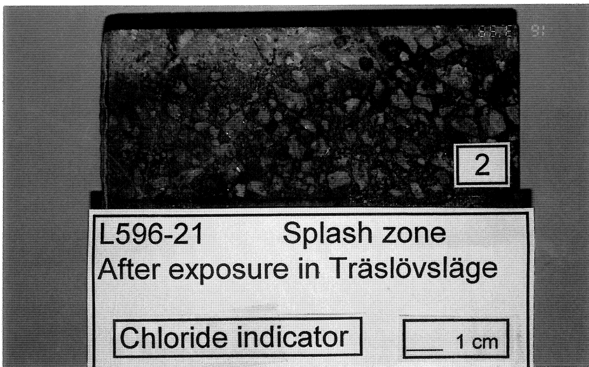
Photo 10. Microstructure and chloride penetration in concrete corrosion cell. SRPC 5 % SF w/c ratio 0.40, after 2 years exposure in the splash zone at the Träslövsläge Marine Field Station. Concrete close to electrode without filter paper defect.
