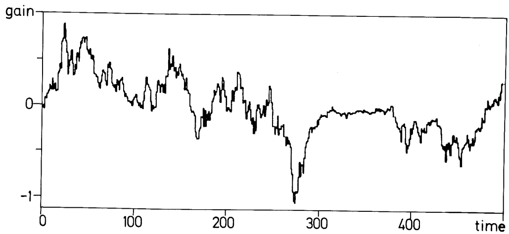
Fig. 18 - One realization of the optimal regulator gain for known parameters.
