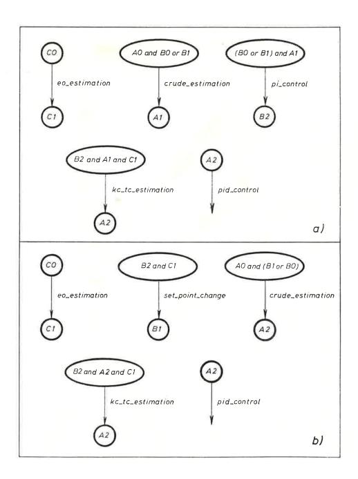
Fig. 1 Partial state-transition graphs for the basic functions of the simple auto-tuner. Graph a) applies when the system starts in state A1, B1, C1 and b) when it starts in A1, B2, C1.
