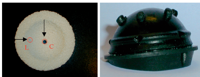
Figure 1. Ceramic acetabular model (L: lateral, C: central) and a 52-mm demonstration Opticup.
