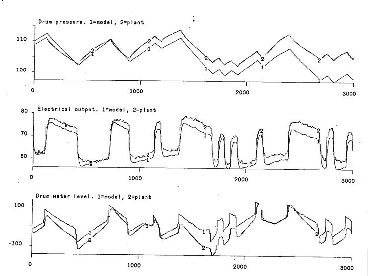
Figure 6. Comparison of plant and model responses, fuel flow changes, high load, simple model.
