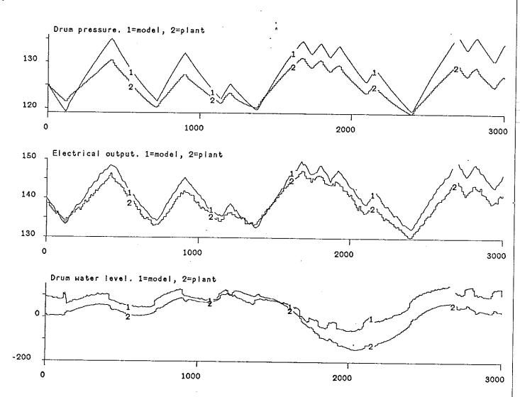
Figure 13. Comparison of plant and model responses, feedwater flow changes, high load, advanced model.
