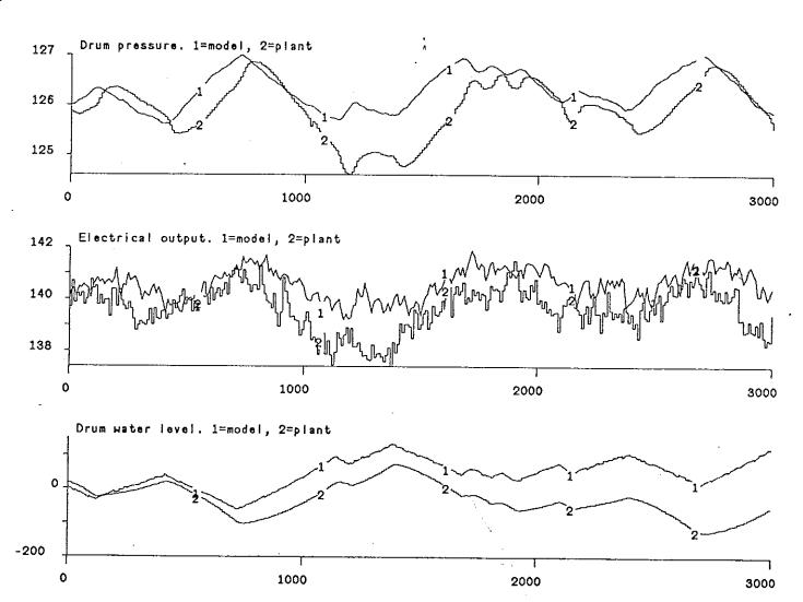
Figure 8. Comparison of plant and model responses, steam flow changes, high load, simple model.
