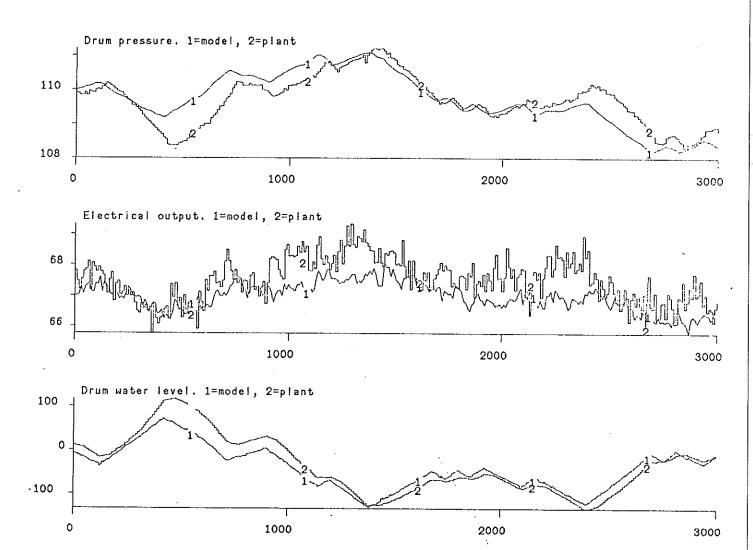
Figure 11. Comparison of plant and model responses, steam flow changes, high load, advanced model.
