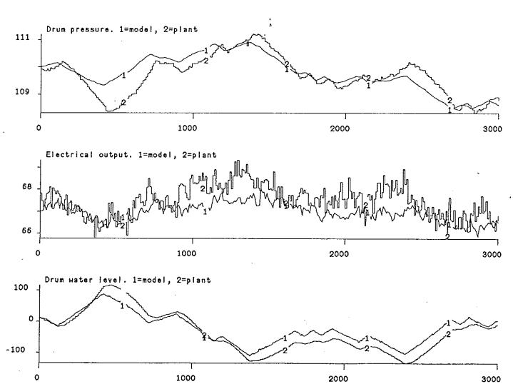
Figure 5. Comparison of plant and model responses, steam flow changes, low load, simple model.
