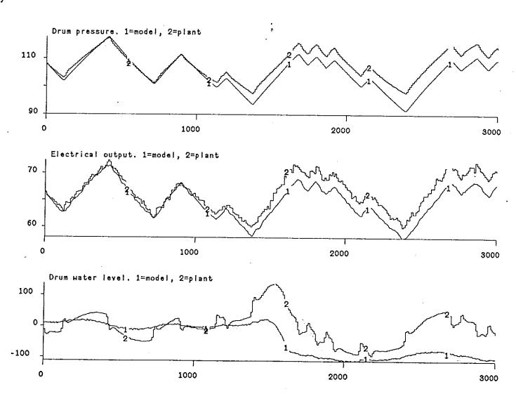
Figure 4. Comparison of plant and model responses, feedwater flow changes, low load, simple model.
