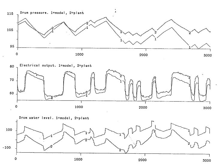
Figure 12. Comparison of plant and model responses, fuel flow changes, high load, advanced model.
