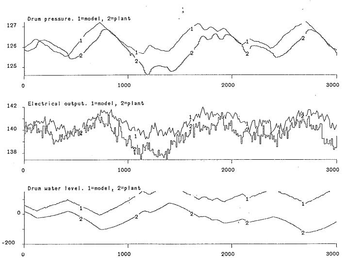
Figure 14. Comparison of plant and model responses, steam flow changes, high load, advanced model.
