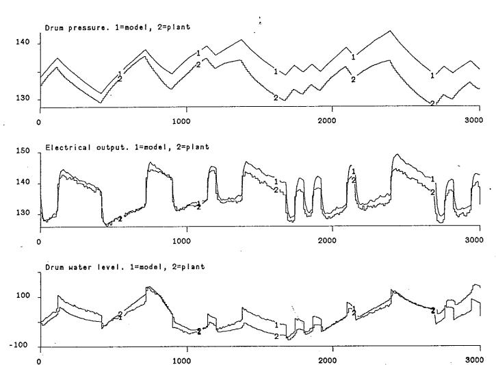
Figure 9. Comparison of plant and model responses, fuel flow changes, low load, advanced model.
