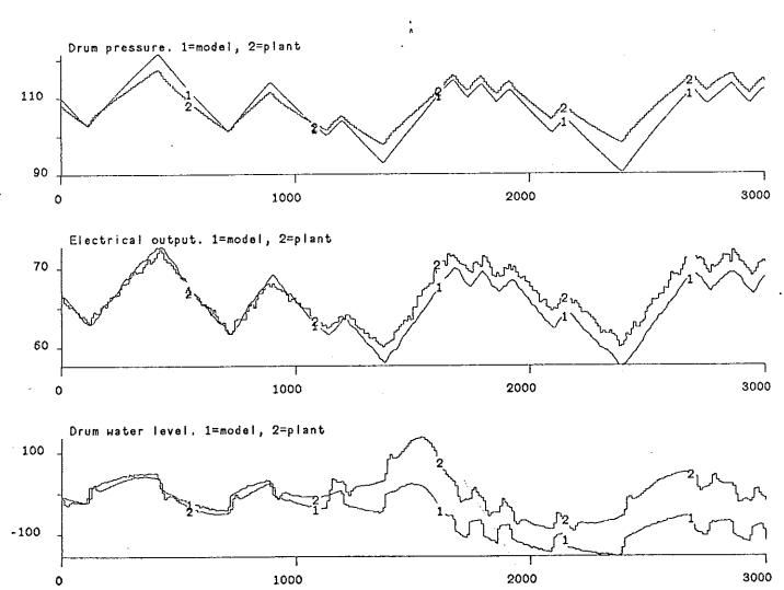
Figure 10. Comparison of plant and model responses, feedwater flow changes, low load, advanced model.
