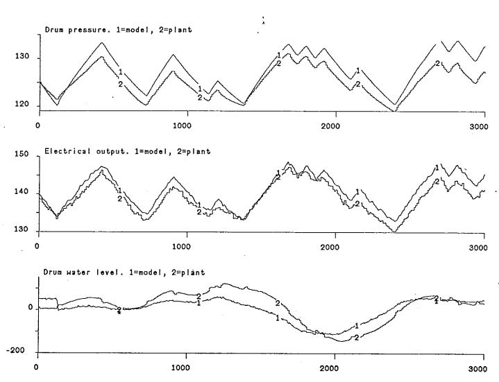
Figure 7. Comparison of plant and model responses, feedwater flow changes, high load, simple model.
