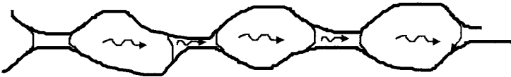
Figure 2-16 Diffusion and capillary suction in the pores. The higher the humidity, the more of the water is transported by capillary suction.
