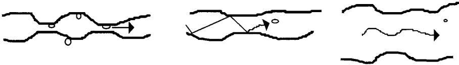
Figure 2-15 Diffusion in dry pores. The wider the pores, the less collision and attraction with the pore walls.
