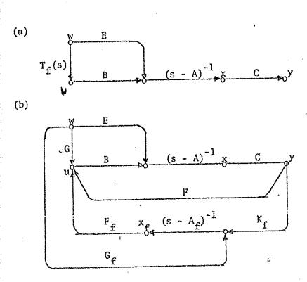
Fig.1. The structures of an external (a) and an internal (b) representatio of a feedback system.
