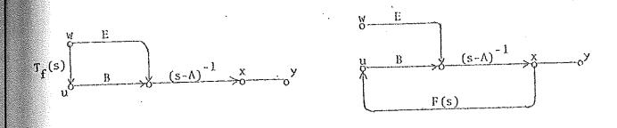
Since F(s) is proper, we can implement the second signal-flow graph by taking a minimal realization of F(s) and connect as the signal-flow graph indicates. This gives a feedback realization of the desired type.
