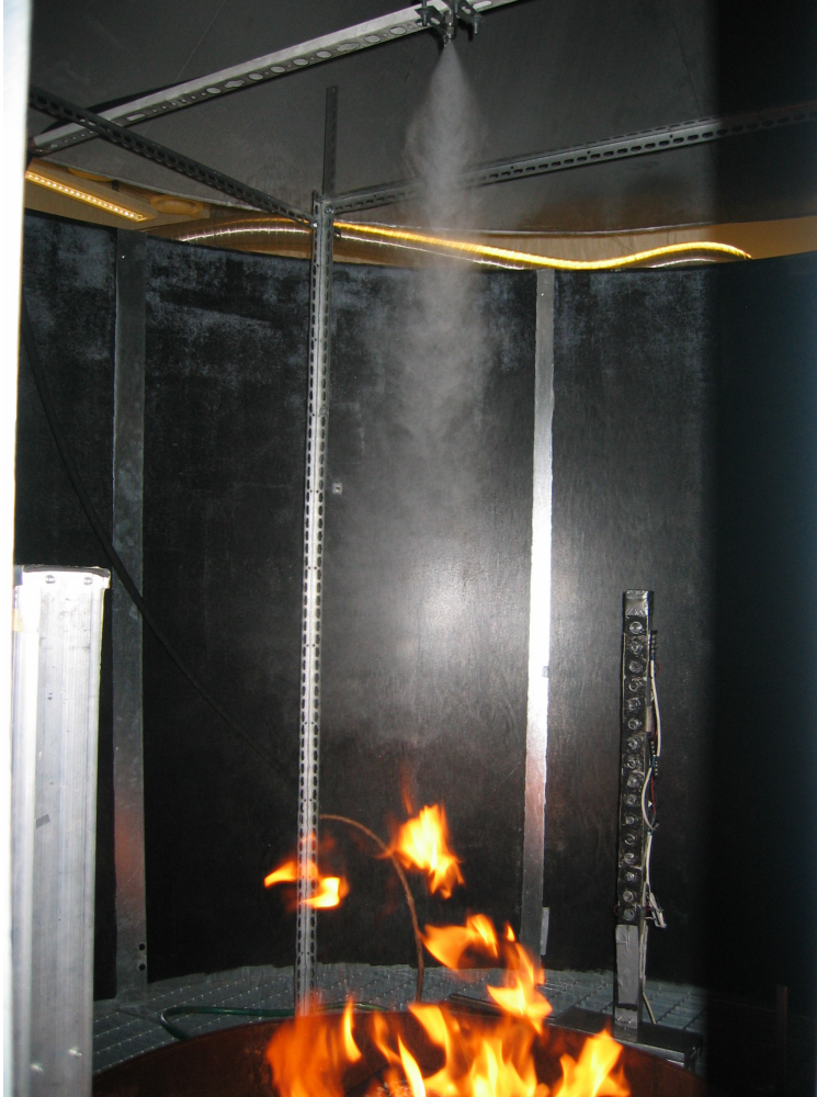
Figure 13. Interaction of water mist and fire during PIV measurements
