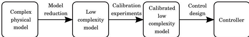
**Figure 1.1** Example of alternative controller development process
