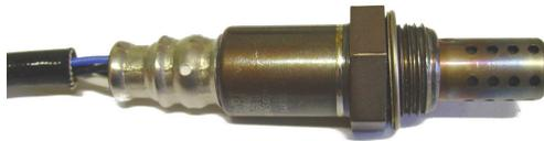
**Figure 3.1** An exhaust gas oxygen sensor
