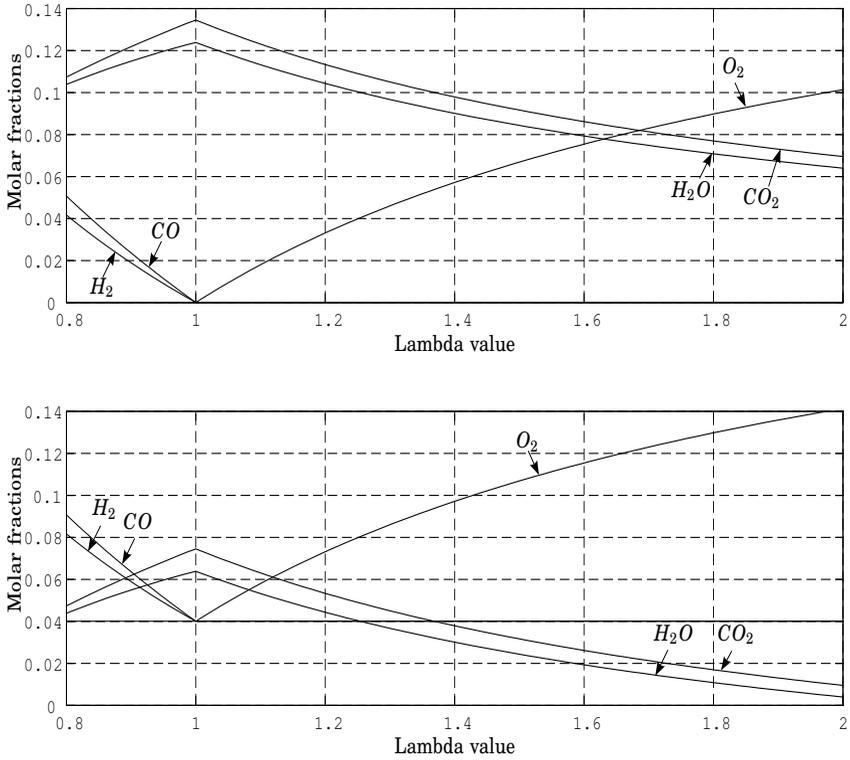
**Figure 3.9** Gas mixtures with the corresponding lambda value
