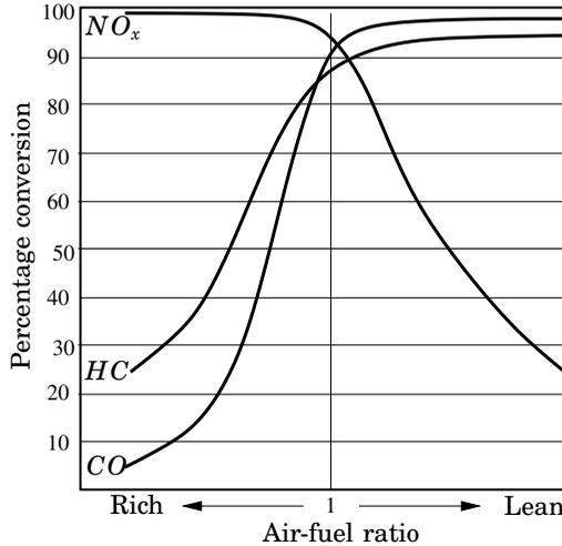
**Figure 4.1** Typical conversion efficiency of a three-way catalyst
