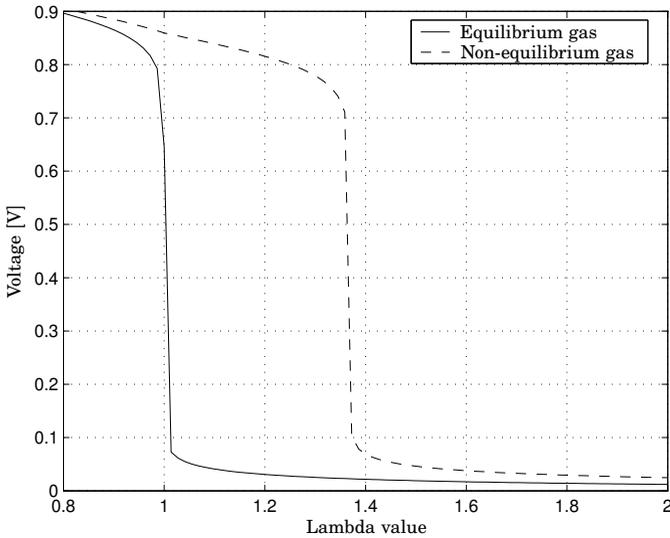
**Figure 3.10** Lambda characteristics simulation
