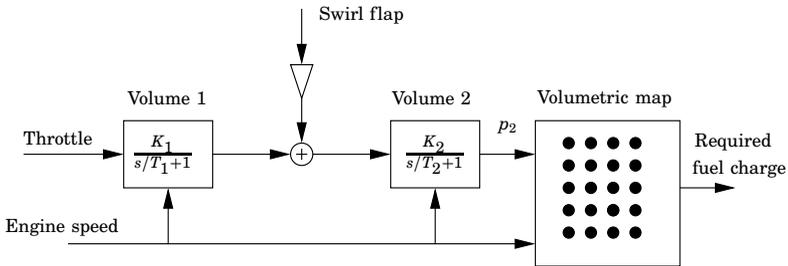
**Figure 4.8** Structure of the heuristically derived model
