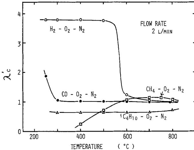
**Figure 3.7** Switch point sensibility to temperature from [Saji *et al.*, 1988].
