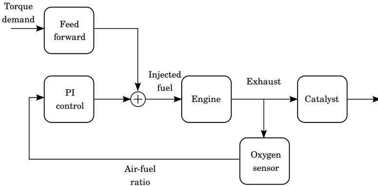
Figure 4.2 A standard air-fuel ratio control scheme
