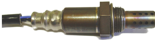
Figure 3.1 An exhaust gas oxygen sensor
