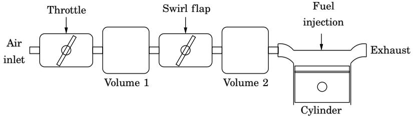
**Figure 4.3** Schematic of the engine air path
