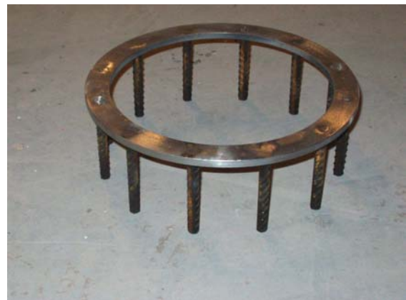
Figure 2.52 - Slump flow measurements, with and without J-ring.
