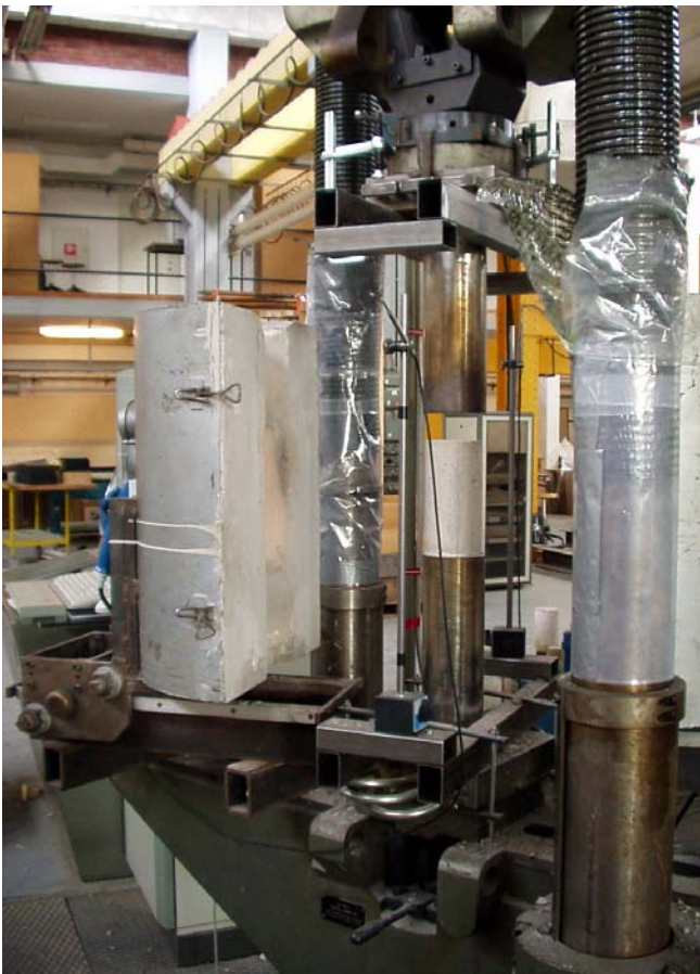
Appendix 3.5 – Details of water -cooled oven with LVDTs before testing
