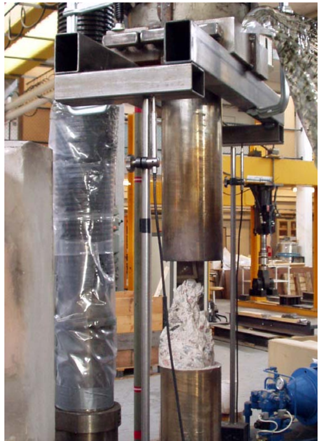
Appendix 3.6 – Details of water -cooled oven with connected LVDTs after testing
