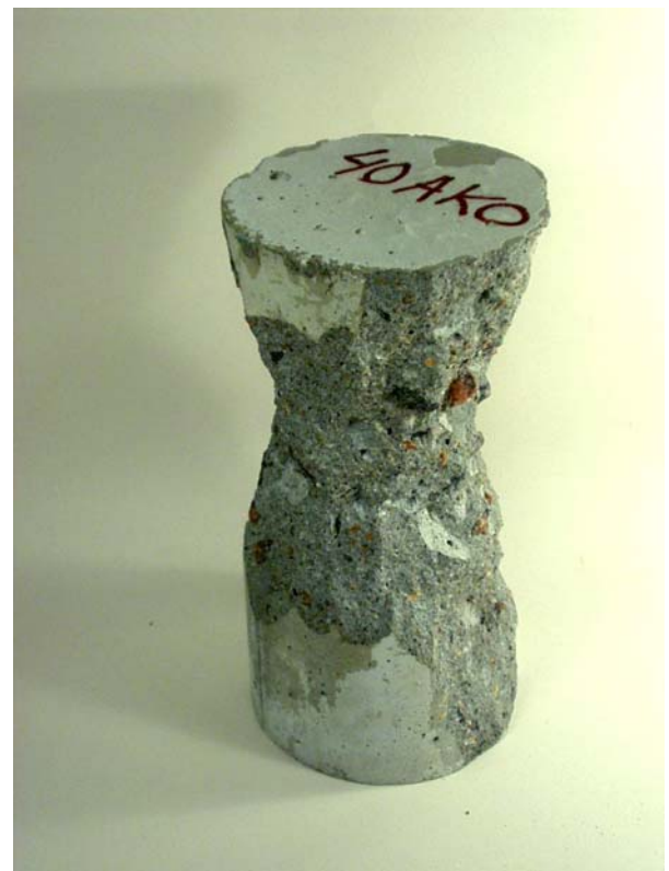
Figure 8.2 – Performance of concrete 40AK0 after heating with 350 °C surface temperature and 185 °C concrete temperature at the time of explosion.
