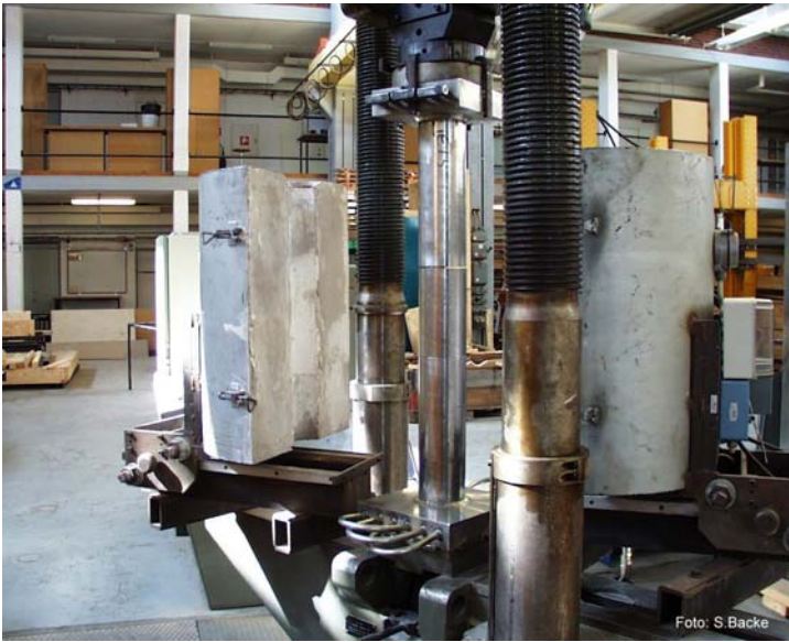
Appendix 3.5 – Details of water -cooled oven with LVDTs before testing
