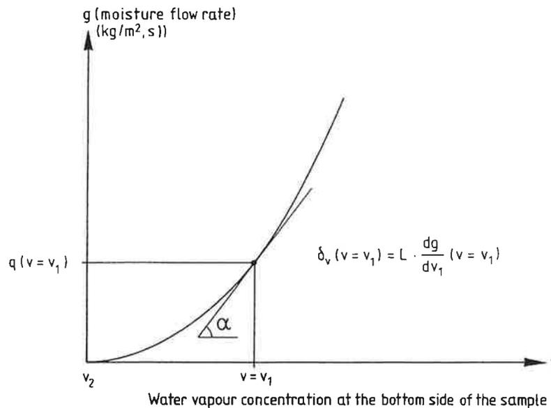
FIG 3 Determination of the moisture permeability.
