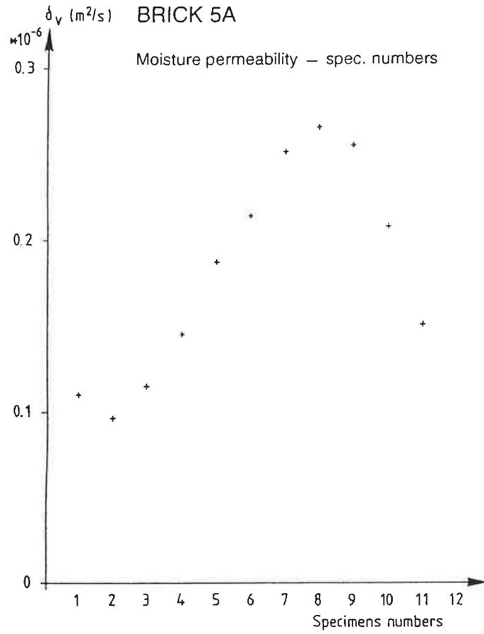
FIG 6 Brick. Moisture permeability for brick 5A.
