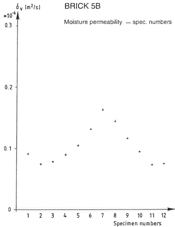
FIG 7 Brick. Moisture permeability for brick 5 B.
