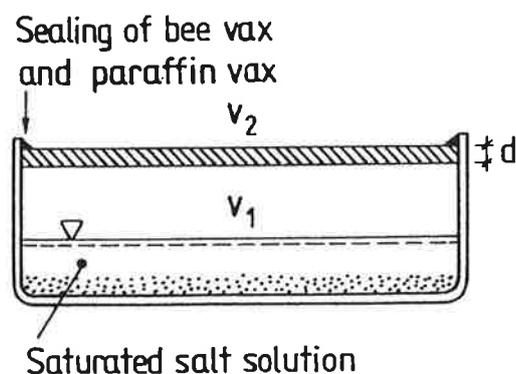
FIG 2 Principle of diffusion measurements with the cup method.
