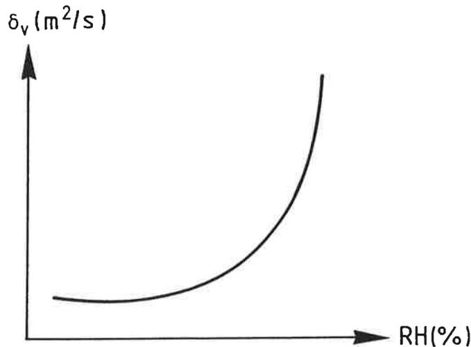
FIG 1. Moisture permeability (with the humidity by volume as potential) as a function of the relative humidity. In principle.
