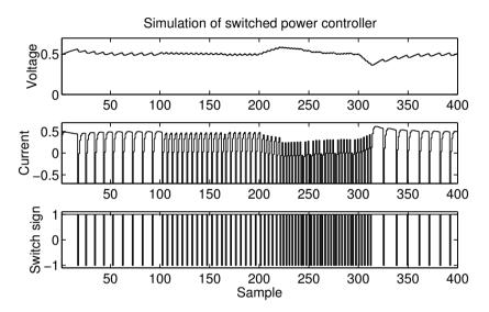
**Figure 5.4** A simulation of the power system example with the obtained controller. At n=100, the load current  $I_{\rm load}$  is changed from its nominal 0.3A to 0.1A, at n=200, to -0.2A and at n=300 back to the nominal 0.3A. The reference value for the voltage is 0.5V
