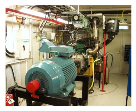
Figure 5.13 Experimental set-up for HCCI engine control
