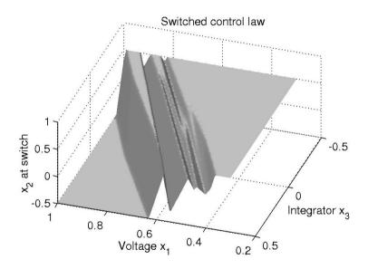
**Figure 5.3** The resulting switching feedback law is monotonous in the current,  $x_2$  (by observation), and therefore it can be plotted in 3D. The plot shows at which current  $x_2$  the switch from s(n) = +1 to s(n) = -1 takes place for varying voltages  $x_1$  and integral states  $x_3$ . Note that the gridding is only for plotting purposes.
