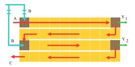
**Figure 5.7** A schematic figure of the reactor part of a plate reactor. The primary reactant A enters from the top left. The secondary reactant B is injected at multiple points along the length of the reactor.  $Y_1$  and  $Y_2$  are measurement signals to the control system, which can control the flow rates of the reactant injections or the distribution of flow rate between the injection points.
