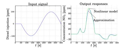
**Figure 5.5** By injecting some extra diesel into the combustion catalyst the  $NO_x$ -levels in the exhausts can be decreased. To the right the responses of a 24th-order nonlinear catalyst model and a first-order approximation to a sine wave diesel injection (left) can be seen. As seen, the number of equations can be significantly reduced without losing much accuracy.
