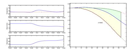
**Figure 5.10** A disturbance acting on a heat exchanger with temperature control. The disturbance has a Feedforward Index of 0.76, indicating that it is suitable for usage in feedforward control action.
