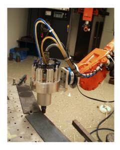
Figure 3.3 Force controlled robot milling (stiff tool and stiff environment).
