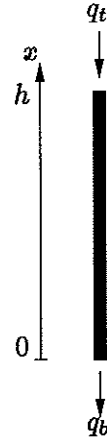
Figure 2 Illustration of the model for the slab temperature (2). The figure illustrates that the rod is heated from the top and bottom with the heat intensity q_t and q_b respectively.
