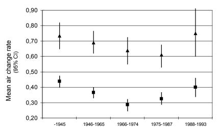
Figure 7. Mean air change and 95% confidence intervals for different construction periods. "■" represents the DBH-data and "▲" corresponds to the Norwegian data by Öie et al. (1998).
