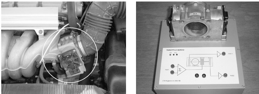
Figure 3.1 (Left) The throttle in a Volvo V70 (99). (Right) The lab process.
