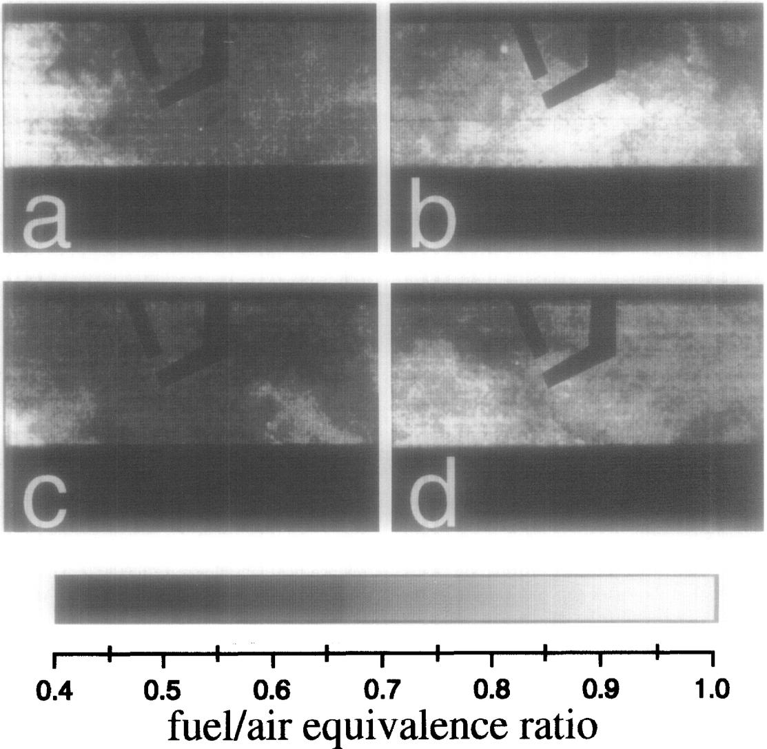
Fig. 2. Four consecutive, single-shot, fuel distributions measured 1 CAD before ignition in the engine shown with the color coding transferred into equivalence ratio. Field of view is  $20 \times 30 \text{ mm}^2$ . Areas in front of spark-plug electrodes have been removed in the images.
