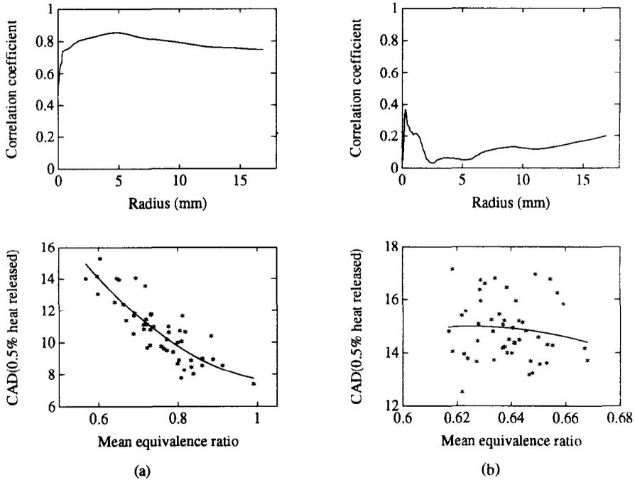
Fig. 3. (a) Inhomogeneous fuel/air mixture. Plot of correlation coefficient as a function of radial distance from spark gap (*top*). The data scatter plot (*bottom*) shows the position (CAD after ignition) where 0.5% of the total heat has been released versus the computed average fuel/air equivalence ratio. The plot is for the radius yielding the maximum correlation coefficient. Best second-order fit is indicated with a line. (b) Similar plots with a highly homogeneous mixture.
