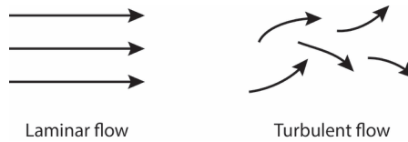
Figure 3. The illustration shows the difference between laminar and turbulent flow. In microfluidics the flow is typically laminar.
