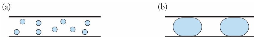
Figure 5. (a) The droplets are small in relation to the channel dimensions. (b) The droplets (plugs) fill the channel width.
