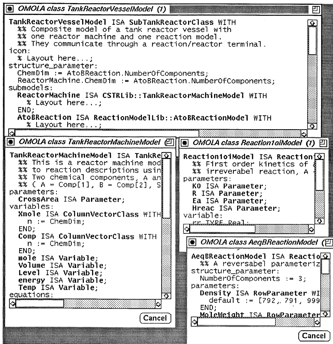
Figure 9.5 The reaction medium and reactor machine decomposition. On the left a part of the machine model and the reactor model are found, and on the top right the composite reactor vessel above the specialized reaction description.
