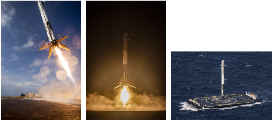
(a) Unsuccessful vertical landing attempt. (b) First stage landing vertically on solid ground in December 2015. (c) First stage landed on autonomous drone ship in April 2016.
