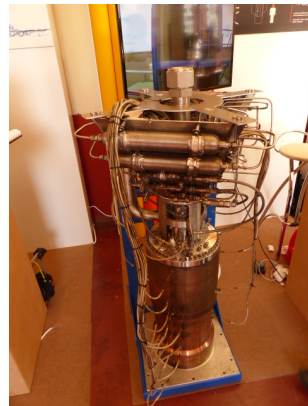
(b) The reusable engine of ARION 1.
