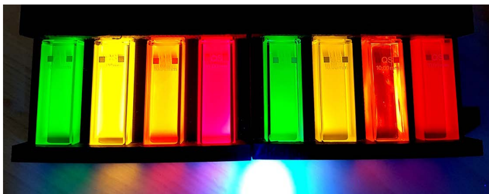
Figure 2. A photo of semiconductor (cadmium selenide, CdSe) quantum dots under ultraviolet light illumination. All the vials contain the same material, but the shapes and sizes of the particles in the solutions differ (e.g., green solution contains particles of size 4 nm x 4 nm x 4 nm, whereas the red one - 6 nm x 6 nm x 12 nm).
