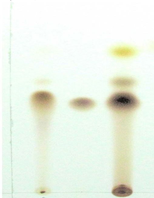
Figure 4. Thin layer chromatogram. From the left BB 0.29 % in acetone, PPD 0.1 % in acetone and oxidized PPD.
