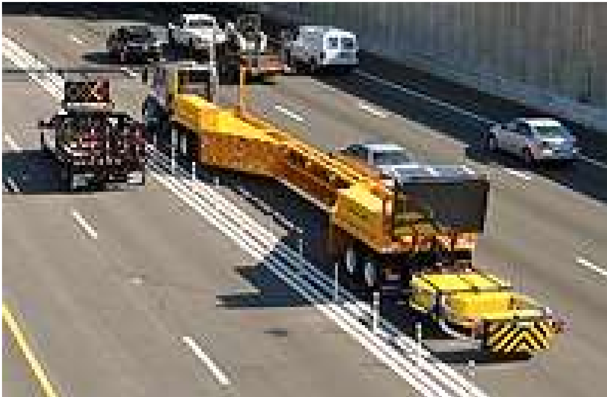
Figure 23. Mobile Barrier Trailer MBT-1. http://www.barriersintl.com/mobilebarriers/images/Photos/day/Mobile%20Barriers%20MBT-1%20Capital%20Beltway%20I-495%20Express%20Lanes/vertical/tb-Mobile%20Barriers%20MBT-1%20Capital%20Beltway%20I-495%20Express%20Lanes%20Maintenance%205.JPG
