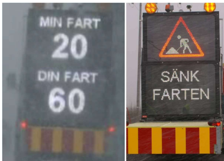
Figure 15. TMA with two Variable Message Signs (text in Swedish). Alternative C with the two phases: 1) "MIN FART" ("MY SPEED") and "DIN FART" ("YOUR SPEED"); 2) road work warning sign and "SÄNK FARTEN" ("REDUCE SPEED" (Sörensen & Wiklund, 2010).
