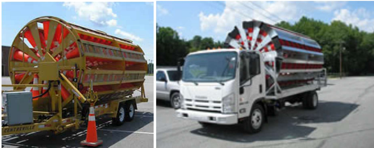
Figure 2. Autocone trailer with magazine for 130 cones and truck with magazine for 500 cones. (SVEVIA, 2014).
