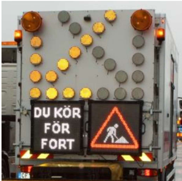
Figure 14. VMS with the text "You drive too fast" (in Swedish) if the driver drove faster than the recommended speed on TMA. " (Sörensen & Wiklund, 2010).
