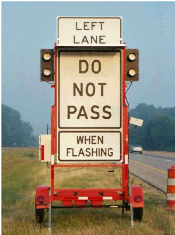
Figure 9. Dynamic lane merger sign (Bushman et al., 2003).
