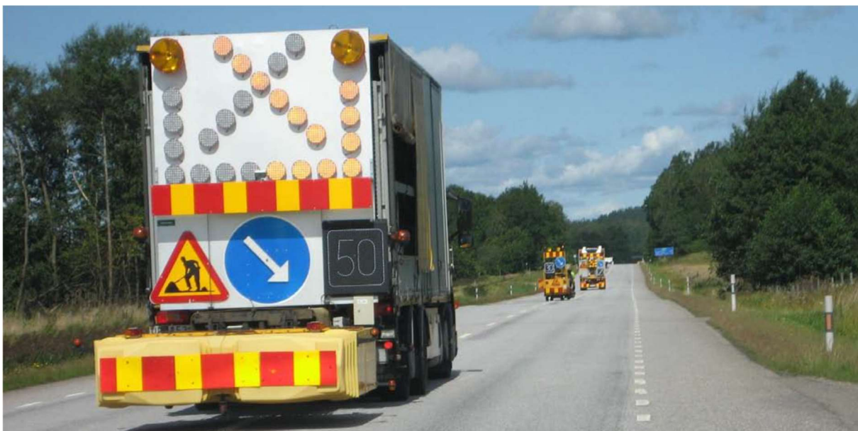
Figure 12. Complementary signage with a Variable Message Sign "Recommended Highest Speed" on road paint vehicles (Persson, 2011).
