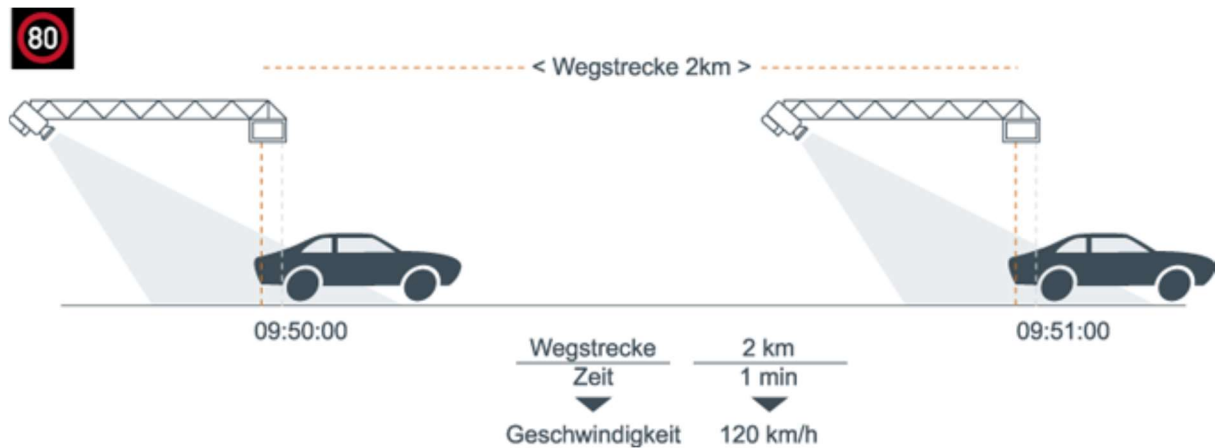
Figure 21. Section speed control (Stefan, 2006).
