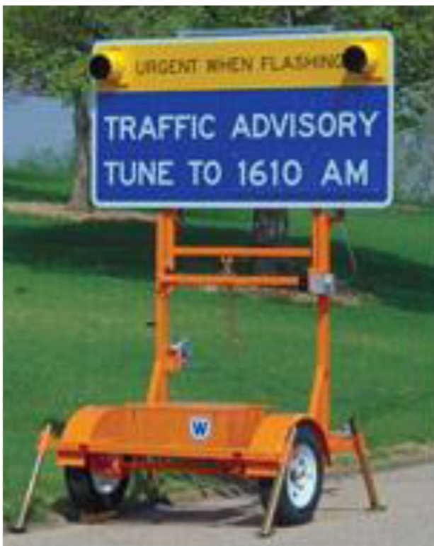
Figure 5. Highway Advisory Radio System (HAR). https://www.google.se/search?q=Highway+Advisory+Radio+Systems&dcr=0&tbm=isch&source=iu&ictx=1&fir=NztKHIMwMMnP3M%253A%252CSUucky9z00lo6M%252C_&usg=__gqBMM_hZZrfKAxZKFSTe8hPjPhA%3D&sa=X&ved=0ahUKEwi43tOi7pPZAhUBZCwKHUQhCBsQ9QEIQjAG#imgrc=P9PI4uXo6EfWnM: )
