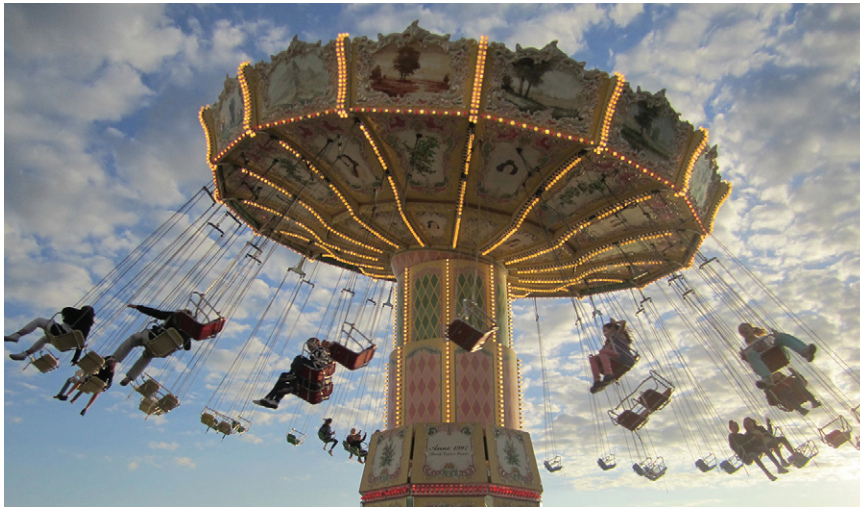
Figure 2. The wave swinger ride, found in many amusement parks, provides a striking example of the equivalence principle: note how empty and loaded swings form the same angle to the vertical. (The wave swinger in the photograph is found in Gröna Lund, Stockholm.)
