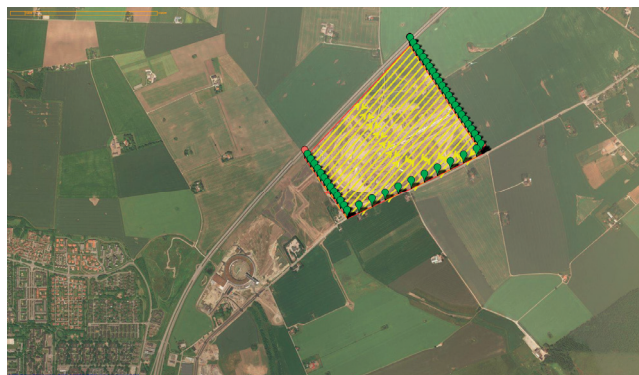
Figure 32. Drone inspection with mobile battery operated 4 \pi dosimeter or/and SiPM alpha/beta/gamma/neutron spectrometer/dosimeter
