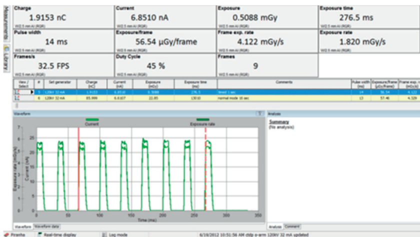
Figure 17. A zoom of a part of the radiation waveform output from a O-arm system.
