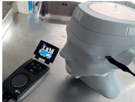
Figure 33. The real time personal dosimeter based on a Si-sensor described in VI. In this application the thin sensor and flexcard is placed inside the phantom where normally only TLD and OSL could be placed.
