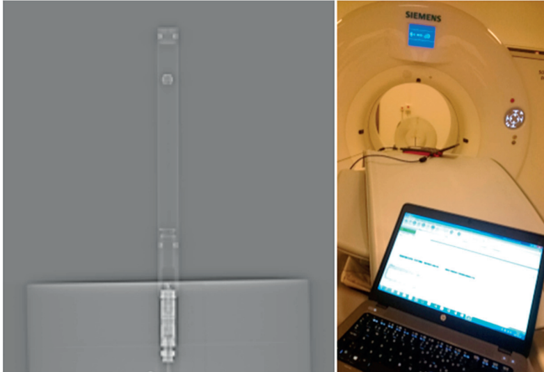
Figure 13. QA CT setup. Scout image and measurement of the dose profile on the first version of the 4\pi energy filter mounted inside the CT assembly probe (Medical radiation physics Malmö).
