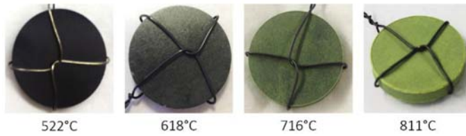
Fig. 2. Tungsten specimens after oxidation in a He-0.5%O 2 gas mixture (2 h).
