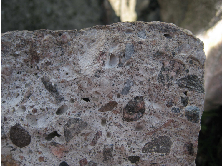
Figure 1: Image showing the strongly heterogenous micro-structure of concrete. The visible pores of the cement paste matrix allow for mass transfer.
