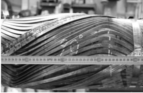
Figure 1: Lateral buckling of armour wires
