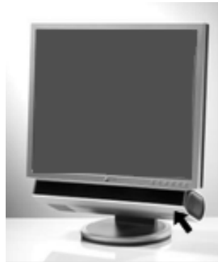
Figure 8: Example of a remote eye-tracker (the arrow shows where the camera is located) as used in Papers II, III and IV.
